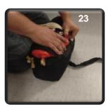
It takes practice to pack quickly and neatly. Every jumper has his own technique to make this easier and you'll quickly develop your own. The whole canopy should be in the bag before you follow your rig manufacturer's instructions for closing the bag, stowing, the lines, placing it in the pack tray, and closing container.
