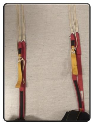
Set the deployment brakes according to the manufacturer instruction of your harness container system or riser manufacturer.
