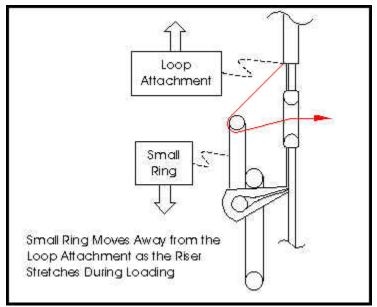
Figure 4: Typical Riser 3-Ring Under Heavy Load
