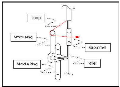
Figure 2: Typical Riser 3-Ring Closing Method
