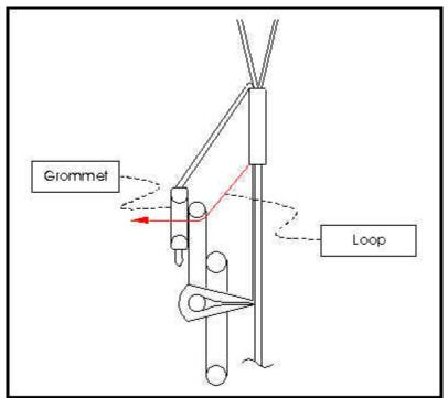
Figure 3: Reversed Riser 3-Ring Closing Method
