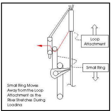
Figure 5: Reversed Riser 3-Ring Under Heavy Load
