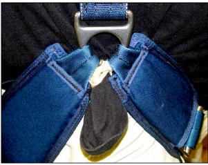
We are currently observing a new trend that involves placing rubber bands on the hip rings of a rig's harness in order to stow one's shirt and keep it from riding up in free fall or under canopy.
