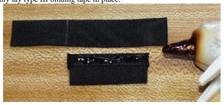
d. Fold short end over and lightly hot glue back side into place.
