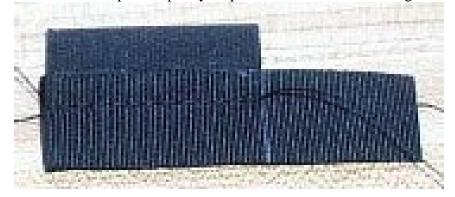
c. With a crafts hot glue gun, run a thin bead across the binding of the elastic keeper and firmly lay type III binding tape in place.
