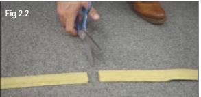
NOTE: Be sure your scissors are very sharp. We suggest you practice on a lower section of Kevlar (below the disc). The cut will be more accurate when the Kevlar is under tension.
