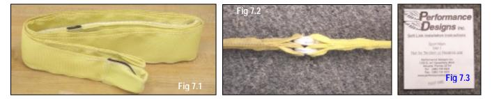
**8.** Insert the center line into the Kevlar bridle. Check the center line length by extending the Kevlar drogue bridle assembly completely. The center line knot should be 1"– 3" (Fig 8.1) from the guide grommet when properly **tuned**. Lengthen or shorten the center line accordingly. Reattach the drogue bridle assembly to the deployment bag.
