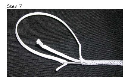
Use the finger trap tool to carefully pull the last end through and out at the  $7 \frac{3}{4}$  " mark
