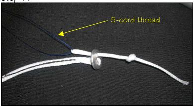
The loop is now attached to the Cypres washer. It is helpful to use some 5-cord thread (pr similar) threaded through the loop to pull it through the small hole of the washer.
