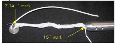
Insert the finger trap tool in at the 15" mark and exit at the  $7 \frac{3}{4}$ " mark as shown.
