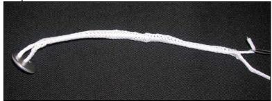
Use the finger trap tool to carefully pull the other end of the spectra line through and out as shown.
