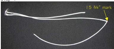
Fold the spectra at the 15 3/4" mark as shown. This will become to end of the closing loop
