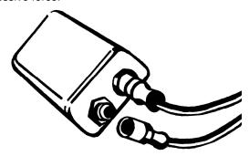
Before installing a new cutter always check the connector for dirt or moisture. If there is anything abnormal please contact your rigger, Argus distributor or the manufacturer.
