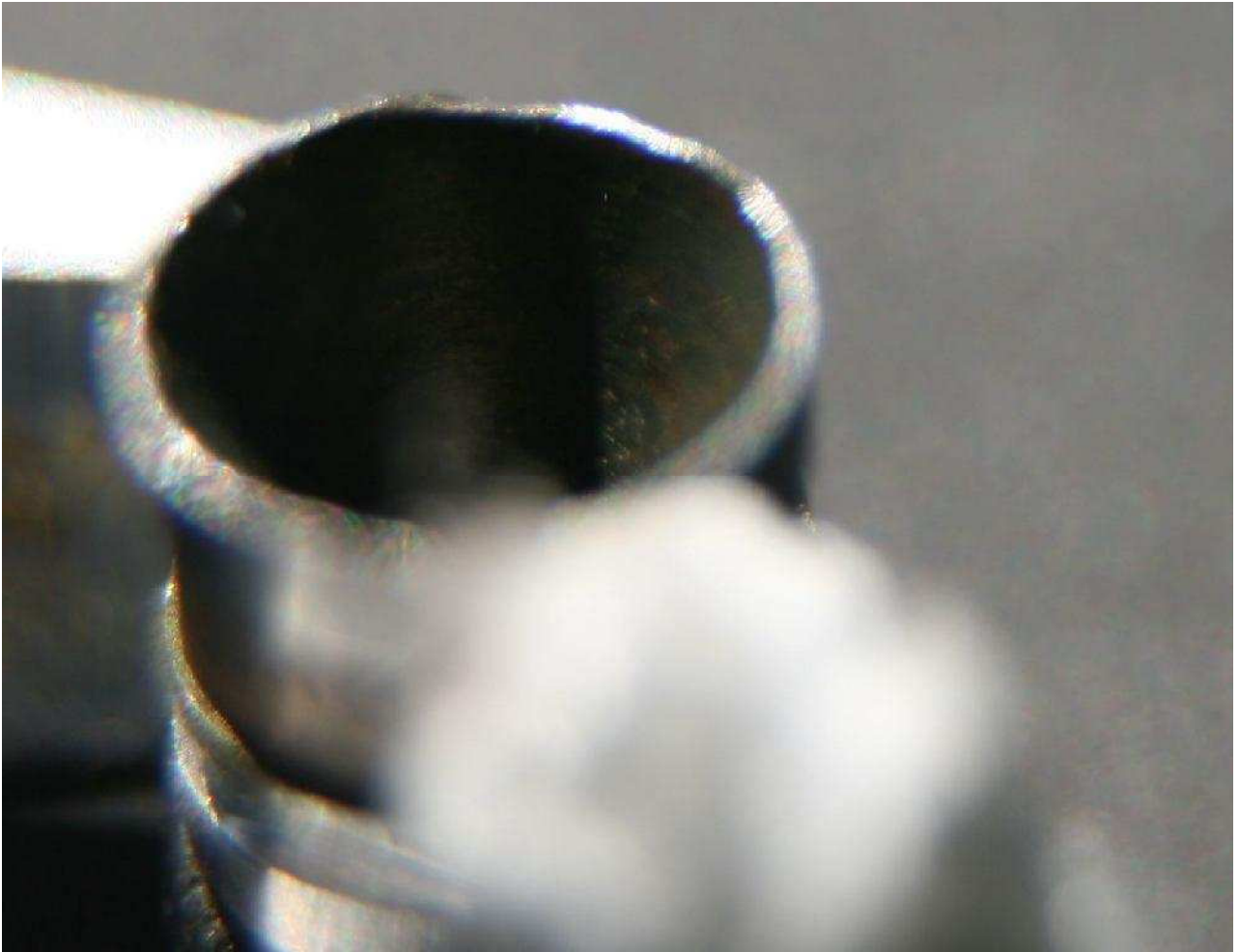
Picture 5: The cutting edge of the blade is damaged
