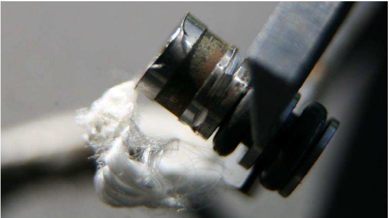
Picture 4: The edge of the bullet cutter was damaged on one side and showed two burrs.
