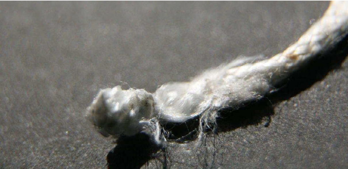
Picture 10: The trapped/pinched loop of the 'San Marcos' cutter
