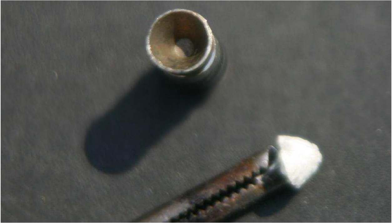
Picture 9: Comparative cutter – Nice molten cone of Spectra fiber (Cutter DOM Aug 2007)
