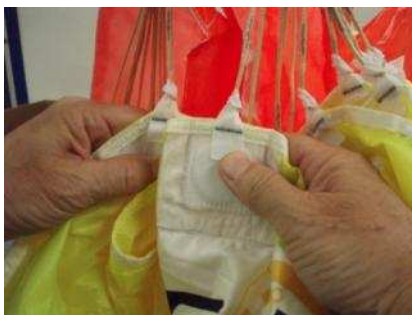
Fig. 15. Take the C1 and B1 attachments and check that they are at the same height.
