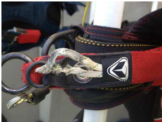
Figure 9: Damaged, Partially Cut
