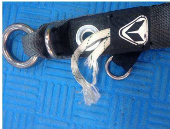
Figure 10: Damaged, Partially Cut
