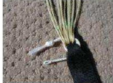
2) Pass the link through the lines and through the riser again, so that the link forms a doubled loop.
