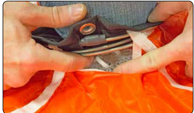
7.13 Folding and stowing the center line.
