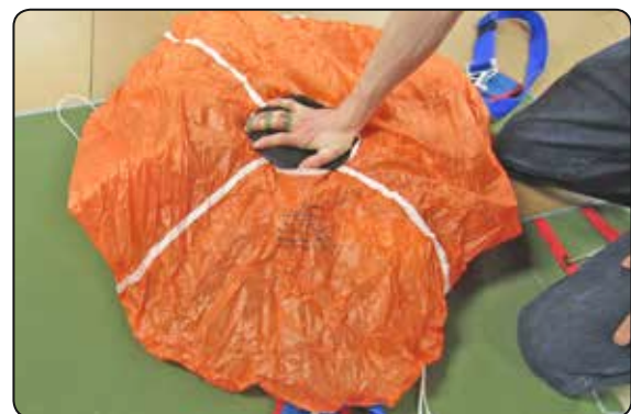
7.11 Compressing the spring.
