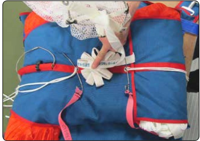
7.9 Stowing the pilot chute bridle.
