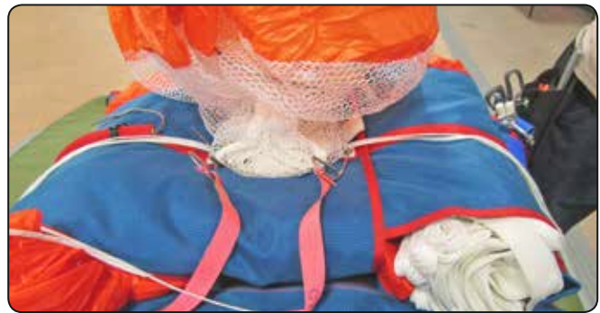
7.10 Setting the pilot chute.
