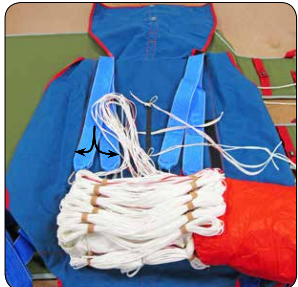
7.2 Placing the diaper.
