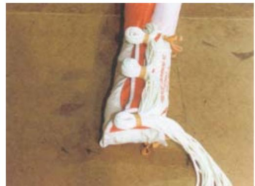
Finish stowing of the remaining suspension lines lengthwise using line loops of no more than 4 cm.
