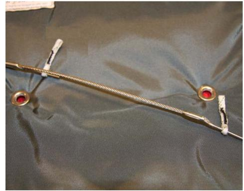
Route both loops through each their grommet in the bottom of the container.
