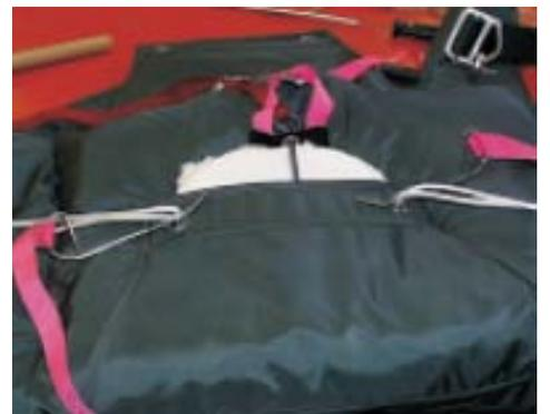
At this stage remove retainer pin and pilot chute retainer in that particular order.
