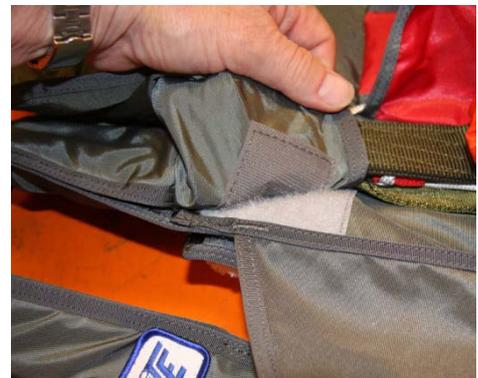
The diaper with the lines to be stowed in a bottom corner of the container, ensuring that it fills out the corner completely.
