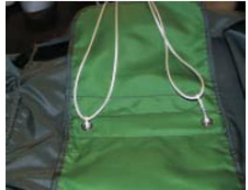
Keep the loops in place in the container by knotting the pull up cords together.
