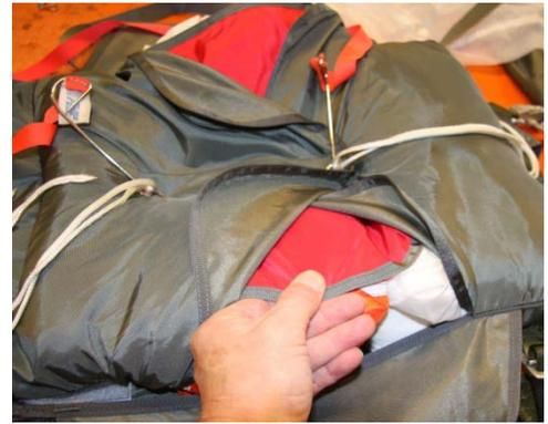
The pilot chute bridle cord is routed out under top flap.
