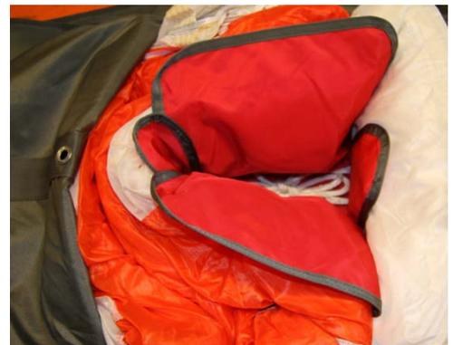
Pull the pull cords up and route them through the grommets in the top and bottom flap. Older models have a slightly longer top flap and are packaged with the bottom flap on the outside.
