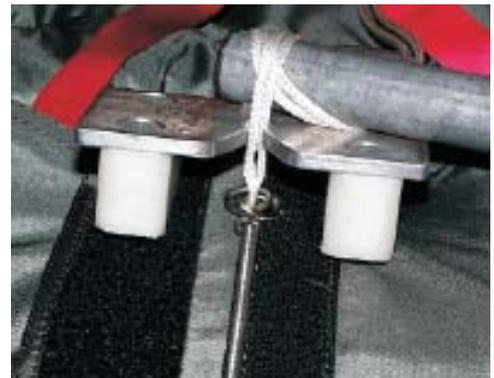
Slowly and carefully remove the pull up cord from the loop. Form a 2m long pull up cord into a large loop with a slip knot. Place this large loop in the other S-hook.
