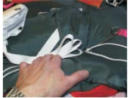
Place the pilot chute on top of the bridle cord. It is **IMPORTANT** that release and warning flags from pilot chute packing retainer and retainer pin are pointing to the right hand side of the container, same side as the side flap with Velcro cover!!
