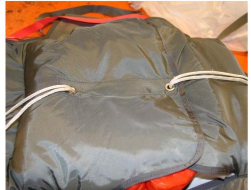
Pull up the loops and insert temporary pins.
