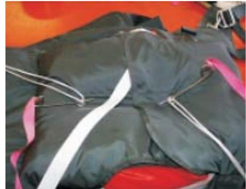
Have the pilot chute packing retainer ready.
