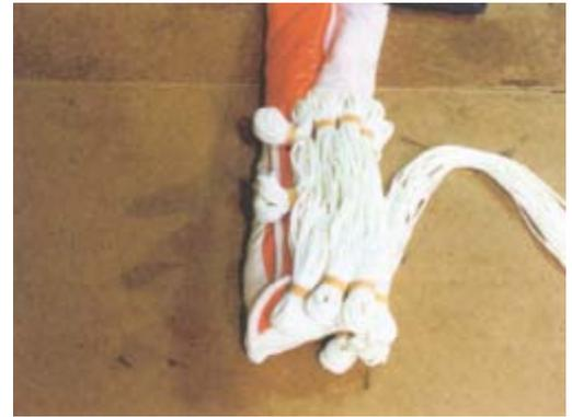
It is mandatory that the pilot chute bridle be installed through both positioning loops on 2 apex vent lines and around all the other vent lines.
