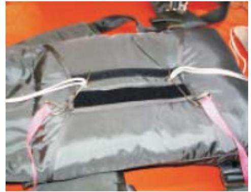
While you hold the closing loop with the pull up cord and the tightening tools, you remove the top temporary closing pin. Carefully install one of the S-hooks in the closing loop.
