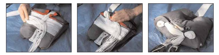
Leave a slack of 40 cm from the free bag to the risers. Remove the strips of loop velcro and mate the velcro at the mouth of the pouch, making sure that none of the suspension lines are trapped by the closure.
