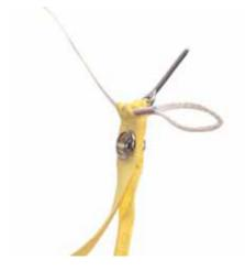
Run the toggle's lower part into the steering line lower loop. Run the entire toggle into the loop and exit it at the top end of the straight pin.
