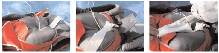
"S" fold the remaining free-bag bridle up and down below the closing loop axis. Route the pull-up cord through the pilot chute and out through the cap. Be careful to not route through in and out the springs. Seat the lower end of the pilot chute on top of the free bag grommet and bridle, keeping the pull-up cord tight.
