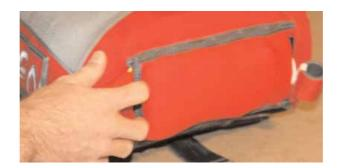
Do not hold the handle, just throw it away. The secondary pilot chute inflates immediatly like a pull-out system and pull the pouch. When in tension the main pilot chute get out from the pouch and open the main container.
