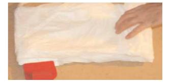
Keep tight the pilot chute when stowing it into the pouch.
