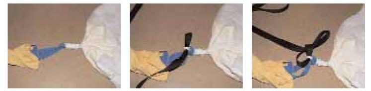
into the main canopy bridle and route the opposite loop end through it. Squeeze the knot to have these 3 bridle attached together.
