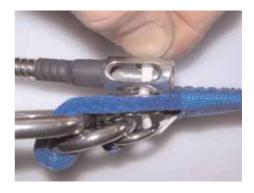
Fit the cable through the white loop and stow the remaining cable. Assembly must be done like on this photo.
