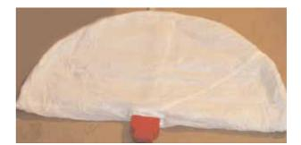
Fold one side of the pilot chute over the opposite side, and then roll it tightly until having cylindrical shape.
