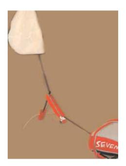
IF YOU DO NOT WANT TO USED THE SECONDARY PILOT CHUTE, JUST REMOVE IT FROM THE SYSTEM. THIS WILL ALLOW YOU TO OPEN THE POUCH ONLY AND YOU WILL HAVE TO EXTRACT THE PILOT CHUTE TO HAVE THE CONTAINER OPEN.
