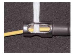
Routing of the white loop through the riser's grommet. Running of the white loop through one of the little round window.
