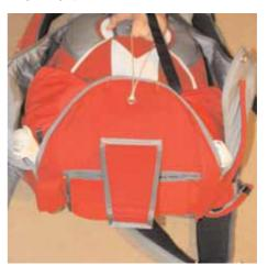
Pilot chute bridle must be route out toward the upper right side. Closing flap order is: -Bottom -Up -Left -Right
