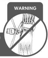
NOTE: It is recommended you replace the Alinks with every new lineset. Check the Alinks for excessive wear and tear, and replace when necessary. It's important to secure the tab in the webbing pocket by tacking the Alink in place with a single stitich of tacking cord through one side of the riser, and knotted in the middle.
