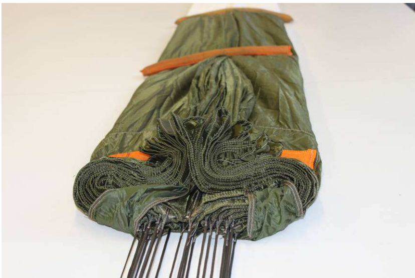
Fig. 14 Parachute canopy folded in thirds
