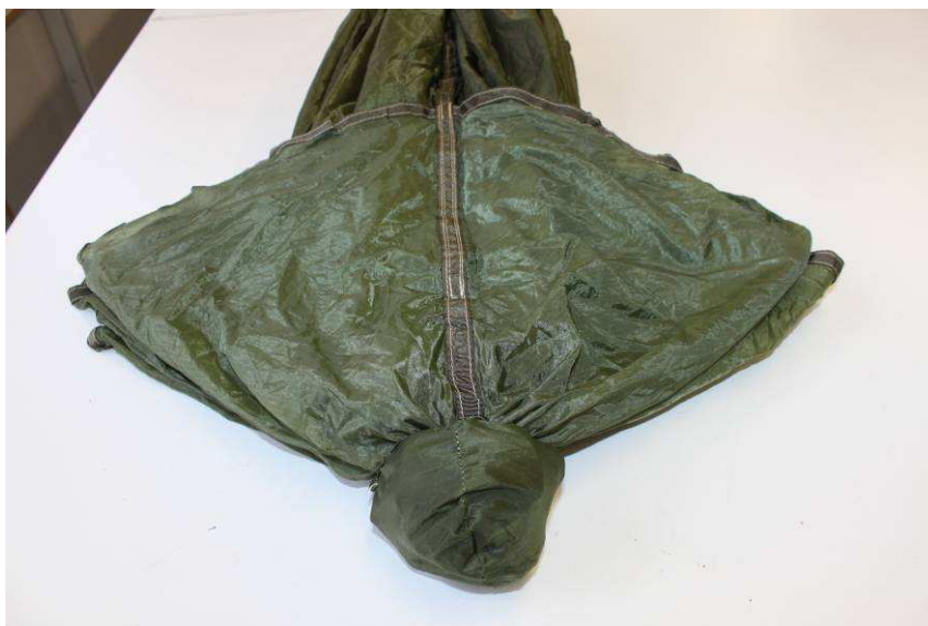
Fig. 15 Inlaid pilot chute
