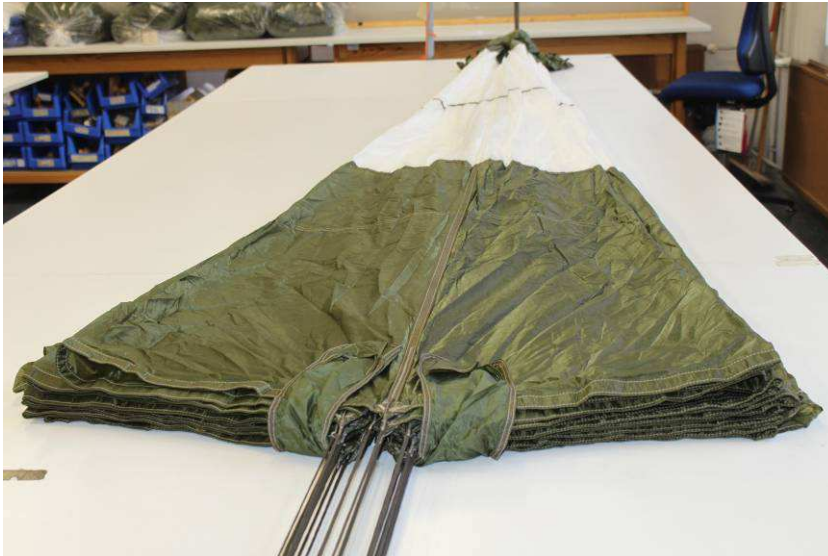
Fig. 13 Inlaid skirt retainers
