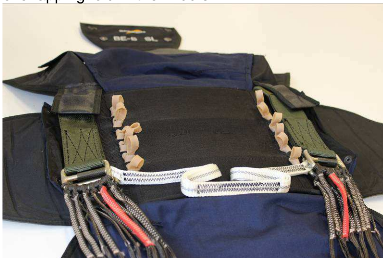
Fig. 16 Inlaid connection harness
