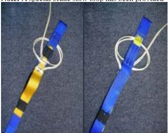
in the top rear of the riser. This loop is for routing the excess steering line. (See Photograph)
