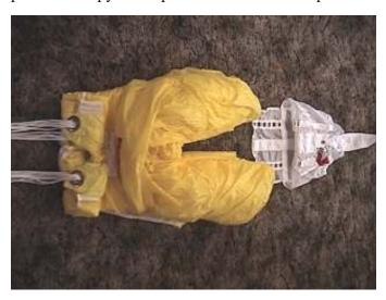
bundle to resemble the bag, prepare the bag and install the canopy into it. The canopy must be folded to mimic the length, width and thickness of the container.
