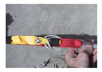
Excess line stows neatly, and releases with "normal" pull force.
