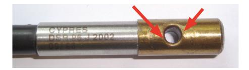
CYPRES cutter in poor condition. Can be repaired by a qualified rigger using fine emery sandpaper. Sharp scratches and sharp corners can be smoothed out and removed especially on both sides around the loop-hole.
