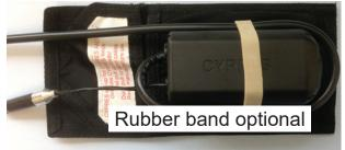
make sure that the cables are not twisted and the big display cable is laying on top of the small cutter cable, to avoid any cable breakages.
