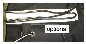
the container bottom. This is optionally and it must be assured that the cable will stay inside this channel at all times and does not interfere with any function of the reserve / container system and deployment.
