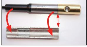
place cutter exactly as picture shows and hole upright in enforcement body
