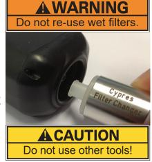
absorbent soft cloth. Remove the old filter from the filter changer by pushing with your finger or with the eraser end of a pencil. Discard it.
