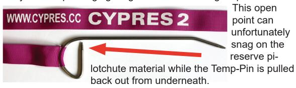
To avoid damages on reserve pilotchutes, you can cover up this part using a 4 inch piece of webbing and attach it like shown.
