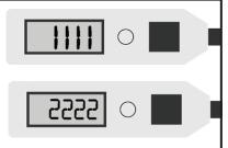
Excessive pressure variations during self test.
