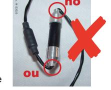
and pull on the cables. So always leave enough slack on all cables.
