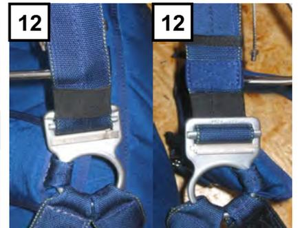
12. The routing of the chest strap, leg straps and adjustability of the main lift.
