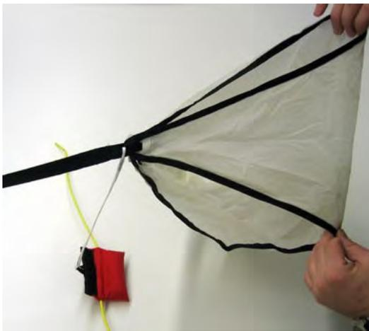
The secondary pilotchute will extract the main pilotchute.
