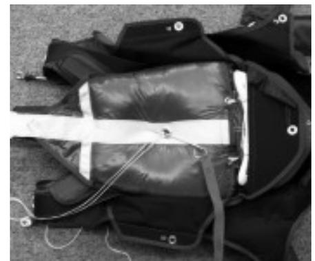
Close flap #1 Route pullup cord through cutter. (Cutter location is on flap #1 or flap #3)
