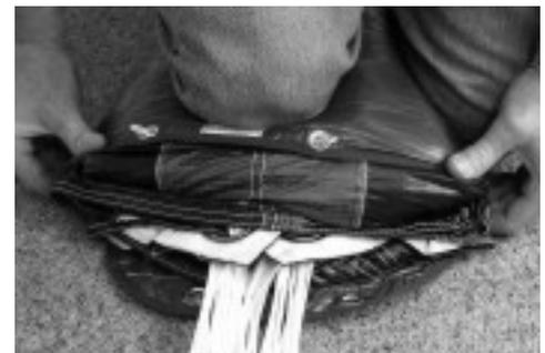
Close the mouth of the bag by performing 2 locking stows. The bite of line should be 2" in length
