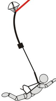
On static line jumps with pilot chute assistance only the static line remains to the aircraft. Less wear on the equipment.
