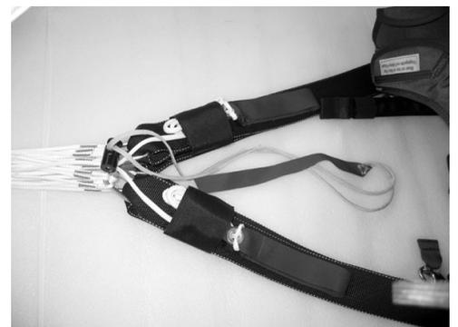
Prepare the freebag by utilizing a Locking cord and Velcro protector strips on The line-stow pocket
