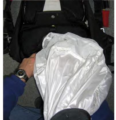
The material of the pilot chute is compress between the springs.
