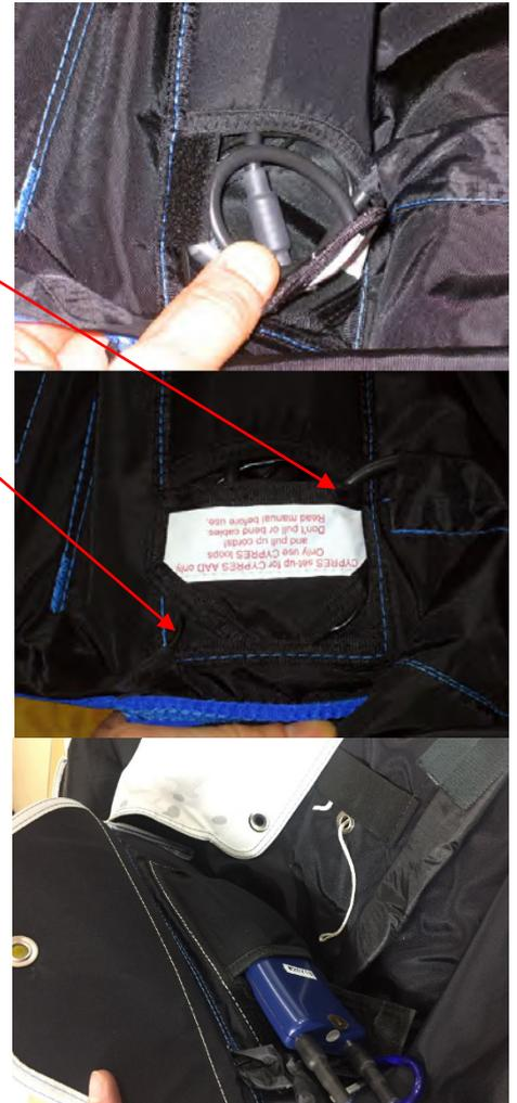
The main pin cover has a built-in safety feature. In the event of an entanglement, the pin cover flap will release.
