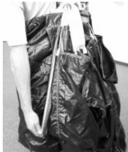
Lay parachute down and recheck nose cells
