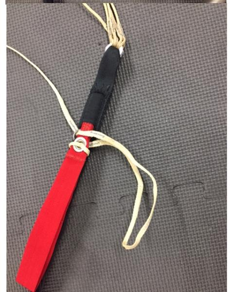
Stow the excess steering line in the keeper on the
