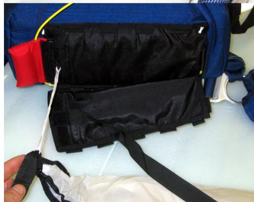
Pack the secondary pilot chute via a series of triangular folds.
