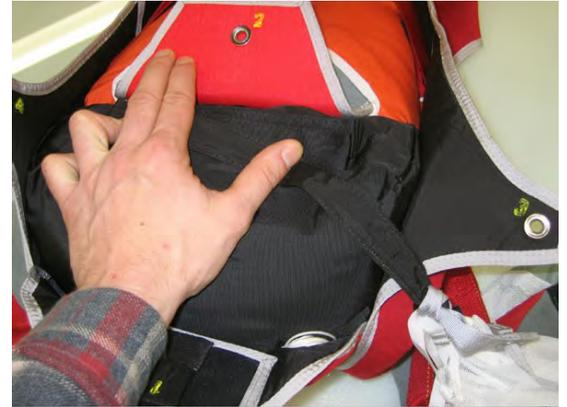
Compress the pilot chute material
