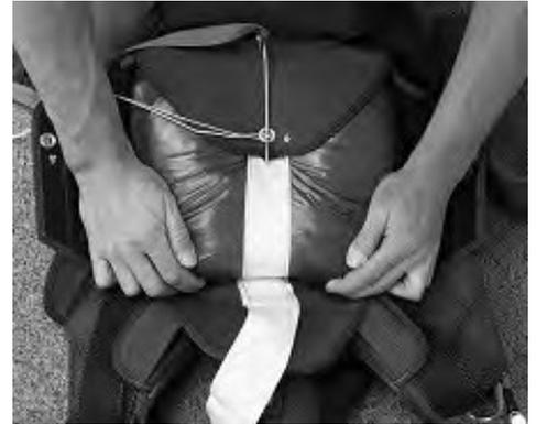
S Fold the bridle across the top of the bag in 5-6" Folds leaving 6ft of bridle to pilot chute.
