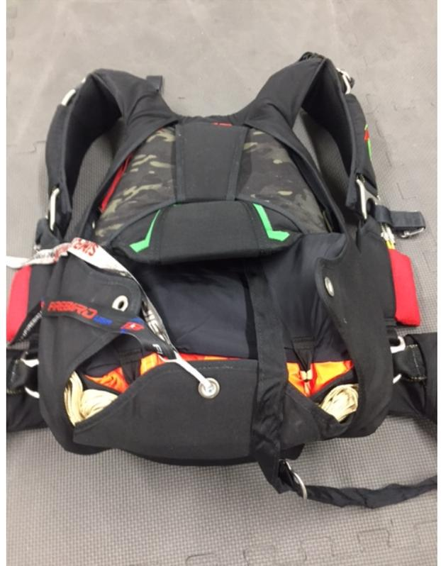
With the closing loop and pull-up cord secured to the bottom flap. Close the top flap.
