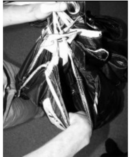
Flake the material between the 'B' and 'C' Lines
