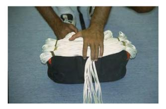
Pull the pilot chute bridle to check that the connection ring of the canopy is not trapping canopy fabric and it is stopped inside the deployment bag by the grommet.
