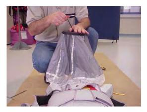
Compress the pilot chute and lock it with the spare locking pin. Pull out the pilot chute fabric from the spring to avoid being trapped.
