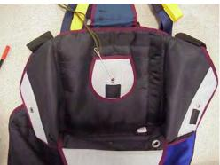
Place the risers on the sides of the harness/container and insert the bag into the reserve container. Using the "T" tool, pass the pull-up chord through the grommets of the deployment bag.
