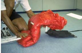
Put your knees over and introduce the remaining fabric inside the last fold obtaining a compact pack. The connection ring of the canopy and the pilot chute bridle must be perfectly visible.
