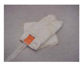
Pass the "T" tool through the grommets on the centre of the reserve deployment bag so that we can pass the closing loop afterwards.
