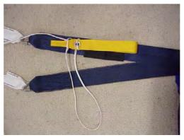
2.- Insert the upper part of the toggle through the brake locking loop and, once inserted, fit the toggle upper and lower part into the pouches above and bellow the guiding ring. Pull the control line until the toggle is in touch with the guide ring.
