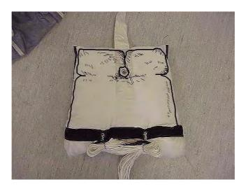
Close the flap of the deployment bag by passing the elastic bands through the grommets. Lock it by stowing the suspension lines in both elastic bands.
