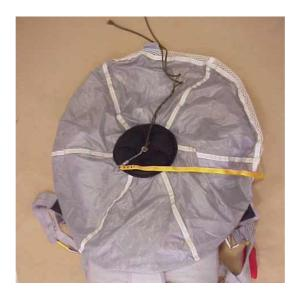
Arrange the fabric of the pilot chute in big folds. It is important that the fabric is not trapped with the sides of the reserve container so that it can exit freely in the case of reserve container opening.
