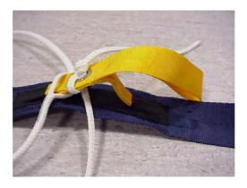
3.- "S" fold the remaining of the control line inside the elastic pouch placed under the same rear riser.
