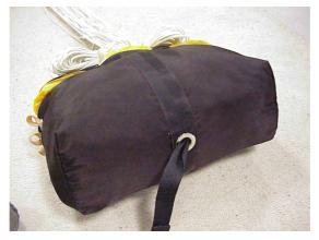
In this moment deployment bag is ready to be introduced into the main harness/container. Introduce main closing loop in the tape of upper part of the bottom of container.
