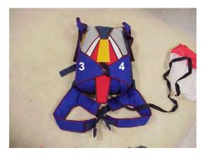
3.- Fasten the Velcro of the pilot chute bridle to the closed upper flap. Introduce the curved locking pin in the closing loop. Remove pull-up chord.
