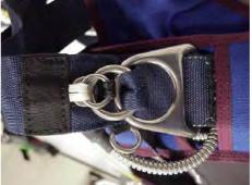
Pass the loop through the grommet of the cut away cable housing. Pass the yellow cable through the loop.
