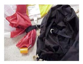
3.-Pull to fix, being careful to avoid friction of pilot chute bridle with union bands/chords when fixing the knot.
