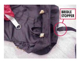
2.- Pass the free loop Nr. 2 of the pilot chute bridle through the connection ring of the main canopy. Next pass the connected pilot chute and deployment bag through this loop.
