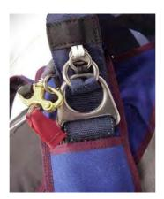
2.- Fasten the Velcro of the RSL with the left reserve riser, aligning both positions.
