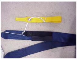
Move the loop along the toggle up to the grommet of the toggle. Pull to fix. Attach the toggle to the velcro on the riser.
