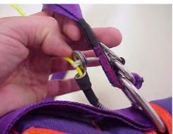
Introduce the extreme of the cable into the corresponding pouch of the rear riser.
