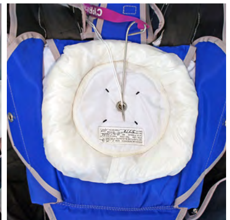
21. Neatly roll the Pilot Chute Fabric up against the outer rim of the Reserve Pilot Chute. Do not tuck the Reserve Pilot Chute Fabric under the lateral closing Flaps #3 and #4.
