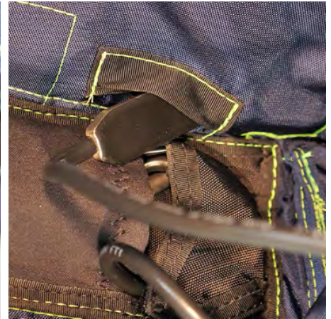
6. Route the AAD Control unit through the Back pad.
