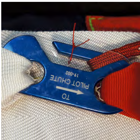
25. Secure red lanyard with one turn of 4 lb. break strength red seal thread.
