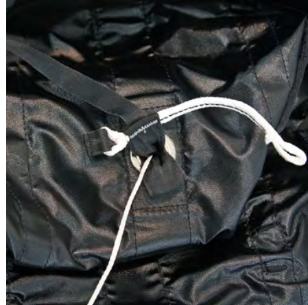
2. Make sure to pull into the D-bag as much as possible to facilitate installing the ALink. Follow next steps to complete ALink installation.
