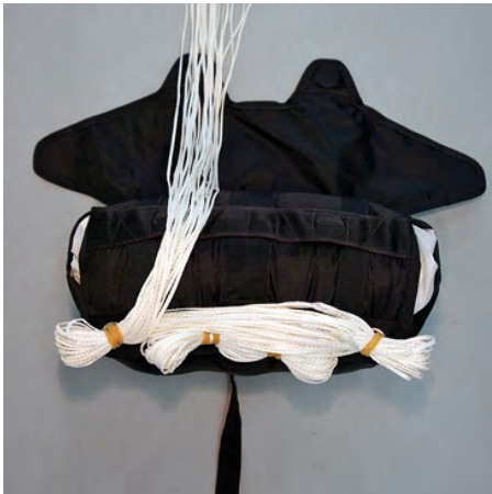
4. Top view of center and outside stows.
