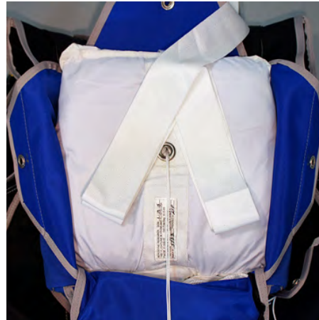
14. Fold bridle in V-shape pattern as shown. Leave a minimum of 4 ft of bridle to base of reserve pilot chute.
