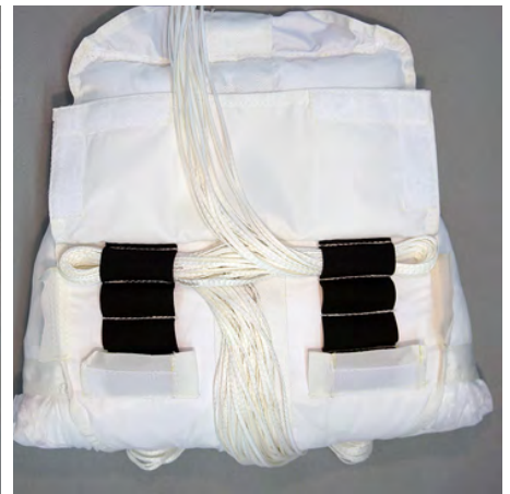
3. Place the next stow in the opposite side top elastic.
