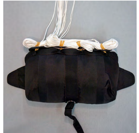
3. Stow the second center stow, then the two outside stows.
