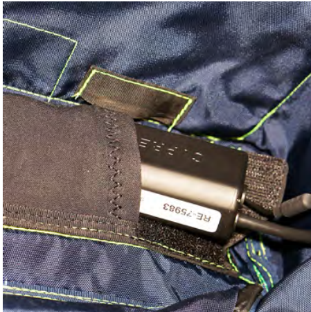
1. Insert the AAD unit into the spandex pocket.
