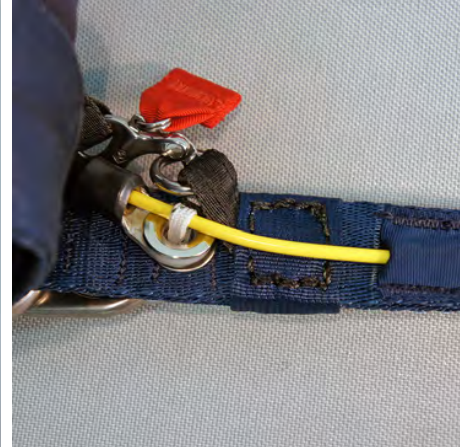
3. Insert the cutaway cable into the Anti-twist Housing.
