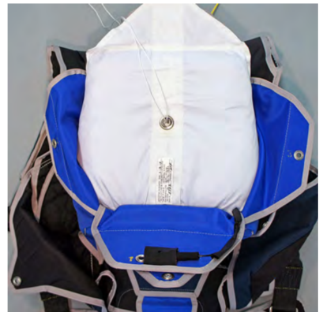
12. Rotate Freebag into reserve container filling lower corners of reserve container.
