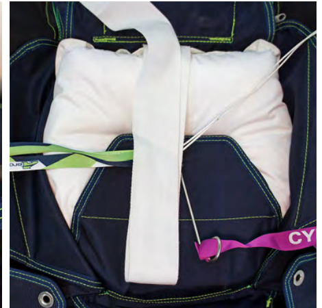
15. Close reserve #1 flap, then place bridle on top as shown.
