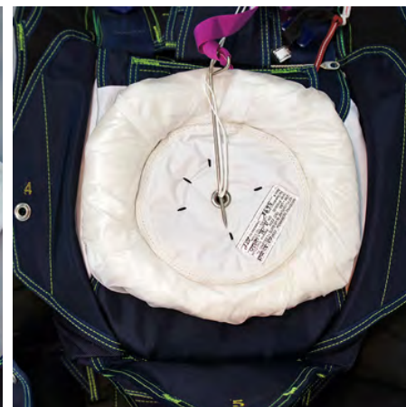
30. Neatly roll the Pilot Chute Fabric up against the outer rim of the Reserve Pilot Chute. Do not tuck the Reserve Pilot Chute Fabric under the lateral closing Flaps #3 and #4.
