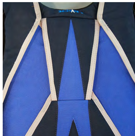
22. Close the final cover flap and tuck the tabs under the #6 flap.
