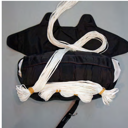
5. Fold the suspension line as shown.
