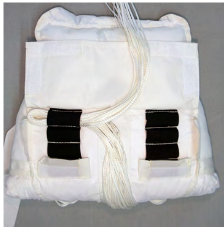
2. Place first stow in elastic keeper at top, opposite side to last locking stow at opening of Freebag.
