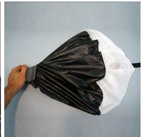
12. Pull the pilot chute to assure it is cocked.
