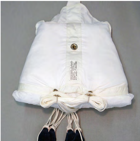
8. Prepare the freebag shape as shown on the pictures above.
