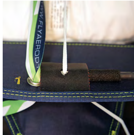
14. To ensure proper AAD activation make sure your reserve loop is threaded through the AAD cutter.
