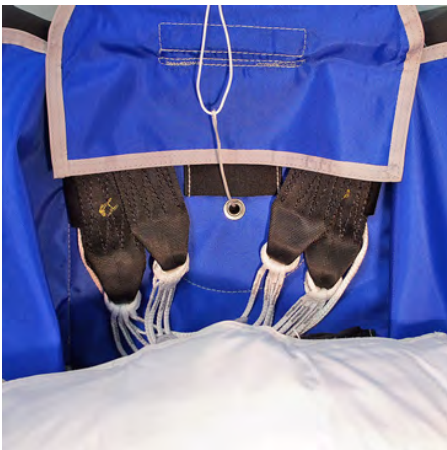
10. Lay the risers flat against the container wall.
