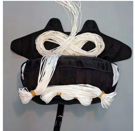
6. Neatly fold the suspension line in a figure of 8 as shown.
