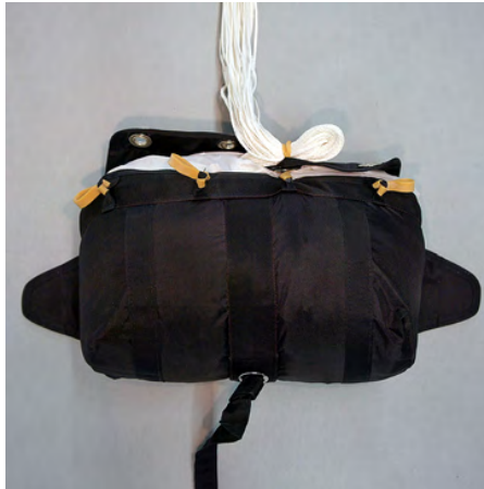
2. Stow the first center stow as shown.
