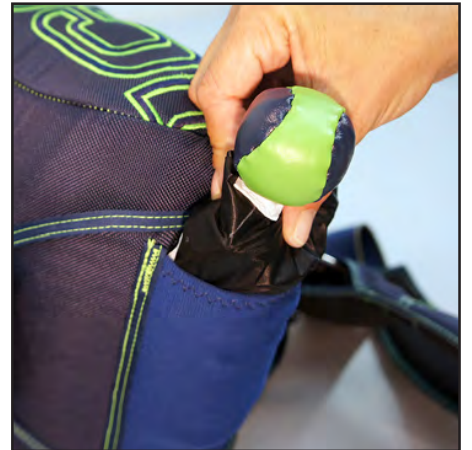
9. Stow pilot chute in BOC Pocket as shown.
