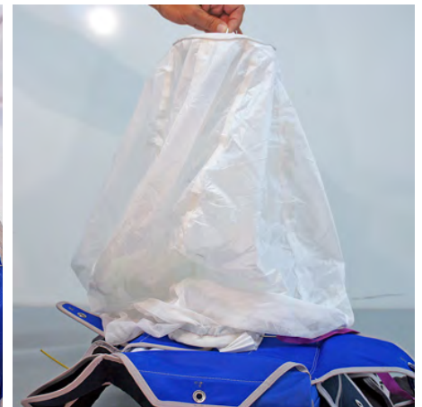
18. Pass the pull up cord cleanly through the pilot chute from bottom to top plate.
