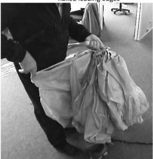
3. Holding the cell inlets firmly, shake the canopy vigorously to clear the fabric from the lines. Then, on one side of the canopy, separate line groups A & B and fold.
