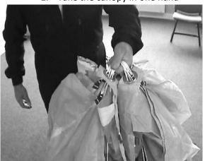
Clear the nose of the canopy by flaking the leading edge. Pull out and count the cells. Align the front edge of the slider with the flaked leading edges
