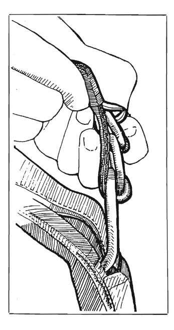
5) Continue threading the white loop through the grommet on the end of the cable housing. The flat side of the cable housing grommet should be against the riser.
