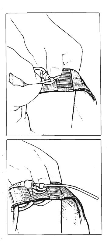
6) Thread the yellow cable through the white loop, making sure the loop isn't twisted. Be careful with the cable so you don't bend it too sharply or kink it. Insert the free end in the channel on the back of the riser.
