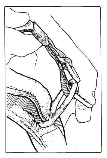
2) With the rings of the riser facing toward the floor, pass the ring on the end of the riser through the large harness ring from above. Fold it back toward the canopy and risers.
