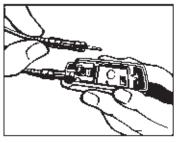
Free the cutter connector and insert the new cutter.
