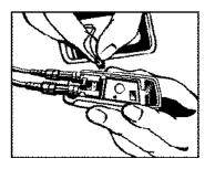
Disconnect the power pack by holding the connector by its small edges. Be careful not to pull on the wires.
