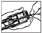
Partially unscrew the printed circuit fixing screw with three complete turns only. Do not remove the screw from the printed circuit board. Do not remove the printed circuit board. (\*)
