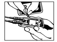
Disconnect the power pack by holding the connector by its small edges.
