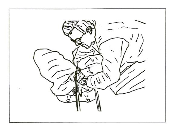
16. Kneel on the grommets of the deployment bag to stabilize it and fold and stuff the ears into the upper part of the bag. Make sure you fill the corners of the bag completed.
