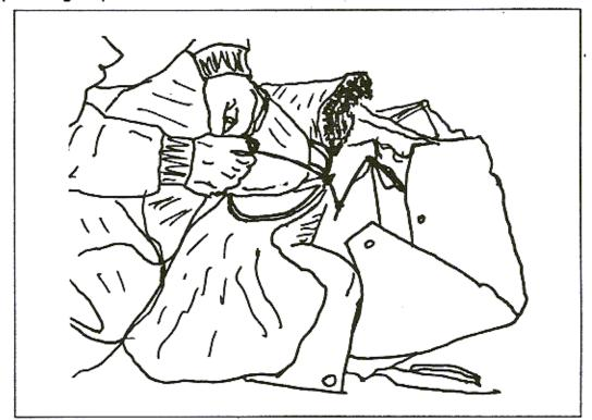
38. Neatly bunch the pilot chute fabric and mesh to each side of the container.
