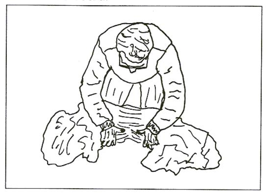
14. Form the ears with the upper portion of the canopy. Keep the nose exposed. Place the molar strap in the middle around the canopy. The strap should go in the middle of the lines group.
