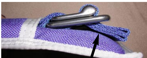
Type 8 buffer No slippage on 0,900 tons
