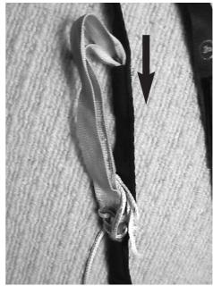
**5** Undo the slider retraction , make sure you have fully stretched slider and that the retractions tabs are pulled firmly against the trailling edge, so that they cannot catch on lines.
