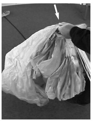
17 Clear each side of the tail and bring them around towards the front (nose) of the canopy. It is very important to make sure that no (steering) lines pass in front of the leading edge (nose), as this may cause a line-over malfunction.
