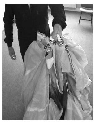
8 Clear the nose of the canopy by flaking the leading edge. Pull out and count nine cells. Align the front edge of the slider with the flaked leading edges.
