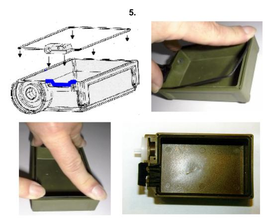
Take the gasket (e) and put into the groove. First press the part of the gasket which covers the cable entrance into place, ensuring that the layer of silicone underneath is evenly spread. Place the rest of the gasket into the groove, taking care not to twist it.
