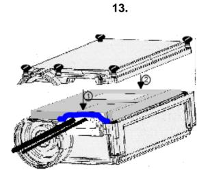
Starting at the cable entrance, place the top of the housing gently on the bottom, making sure that the rest of the gasket remains firmly in place.
