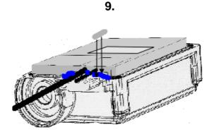
If the CYPRES is a 1-pin model, seal the remaining empty cutter cable routing with the supplied rubber ("blind") stopper.
