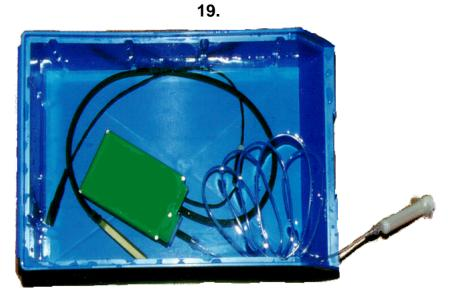
Place the water resistant housing containing the switched off CYPRES and all cables, the cutter and the sealed control unit into clean water. Remove any bubbles sticking to the case by moving the case around in the water.
