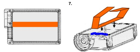
Place the supplied brown strip of capton (appx. 1cm x 18cm) into the bottom case as shown. The strip has to be placed at the edge of the control unit cable. The capton strip must not obstruct the filter pressure entrance point (round metal area).
