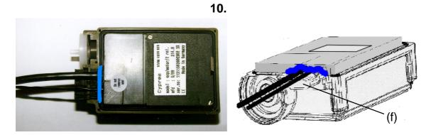
Apply another strip of silicone onto the cables and the gasket as shown.
