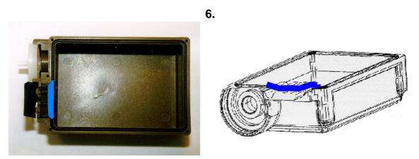
Apply another strip of silicone onto the gasket as shown. Carefully remove any surplus silicone on the inside of the housing.
