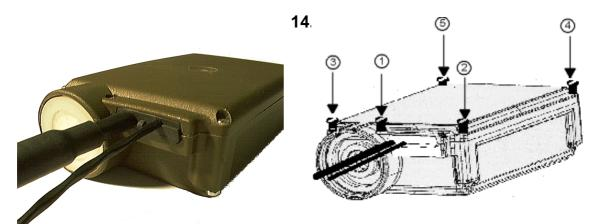
Turn the screws through the bottom housing and mount the nuts. Tighten all screws very gently and evenly. Then begin the final mounting by tightening screws 1-2, then 3-4, then # 5. All screws have to be tight.
