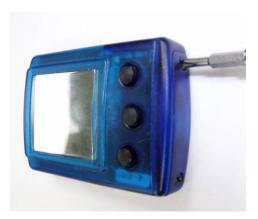
Replace the two screws, but DO NOT OVERTIGHTEN! This can crack the battery cover and cause the unit to lose water resistance.
