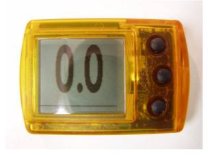
There is also an analog display called the "fun meter". The "fun meter" is a black bar across the bottom of the screen which starts to fill in at 3,000 feet and is a complete solid bar at 12,000 feet. The purpose is to give you a quick indication of where you are between 12,000 feet and 3,000 feet.
