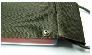
Lay the hand mount across the back of the Neptune. Line up the four (4) holes with the threaded inserts in the back of the Neptune and insert the screws provided, with the washers between the fabric and the screws.
