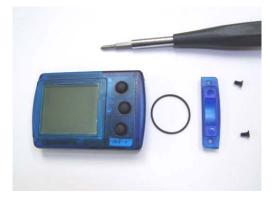
Remove the two screws securing the battery cover using a Phillips screwdriver.
