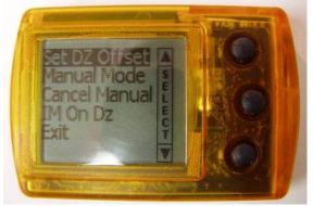
The "*Set DZ Offset*" (Menu > DZ Setup > Set DZ Offset) function allows you to take off at one location and land at another DZ which is at a different altitude. The only function of DZ offset is to enter a number which is either added or subtracted from the AGL altitude that is displayed. The DZ altitude continues to be updated normally.
