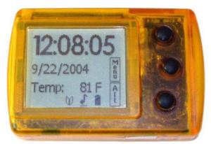
The ground display shows time, date and temperature, and also shows status icons for backlight, logbook, alarms, and battery.
