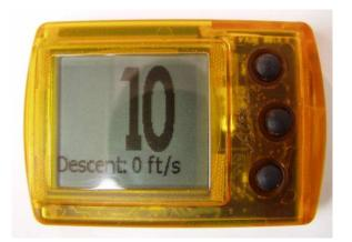
The canopy display shows altitude in feet to a resolution of 10 feet. It also shows rate of descent in feet per second.
