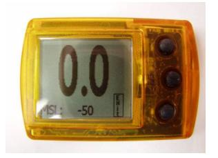
When "Alt" is showed in the bottom right of the screen (in Ground Mode and Climb Mode), push the bottom button to go to the "Altitude" screen. This shows altitude AGL (above ground level) and altitude MSL (Mean Sea Level).
