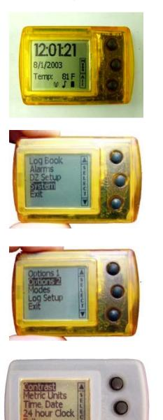
The system starts up in the ground screen. It displays time, date and temperature.
