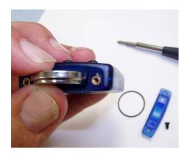
Insert one type Duracell DL2450 (or equivalent) battery.
