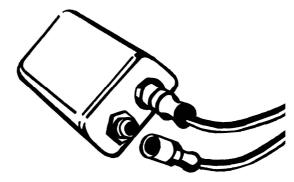
• Before installing a new cutter always check the connector for dirt or moisture. If there is anything abnormal please contact your rigger, Argus distributor or the manufacturer.
