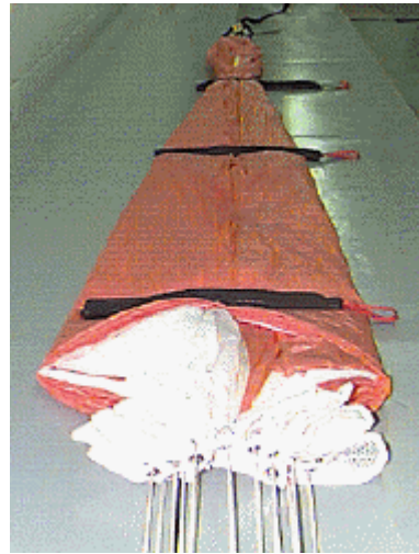
Figures 9 & 10. Fold each individual gore of the canopy 90 degrees, placing the skirt of each gore parallel to the radial seam.
