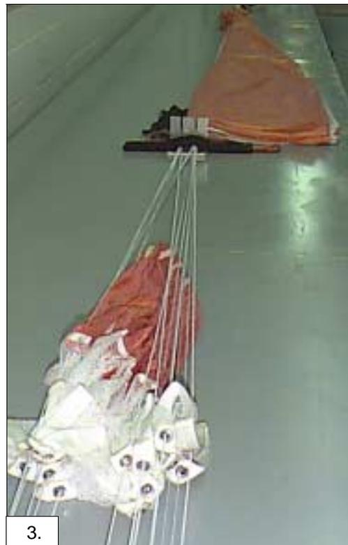
Figure 4. Lay the canopy out with an equal number of gores on each side. This will leave the back center gore (with mesh) on top.
