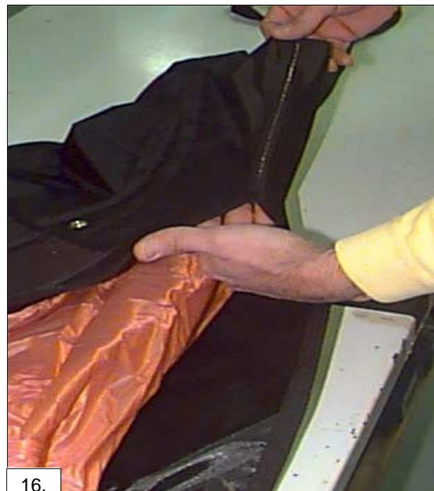
Figure 17. Holding the freebag open with one hand, place the canopy apex up into one corner.
