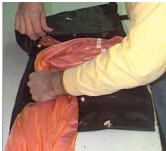
Figure 20. When enough canopy has been S-folded into the freebag to reach the first grommet, insert a locking pull-up cord into the grommet from the underside of the freebag...
