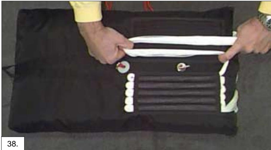
Figure 38. After filling all the flutes on one side, continue stowing the lines in the next set of flutes. Note: As you measure and form the next bight, allow enough line to reach from the last flute you stowed to the first flute of the next set.
