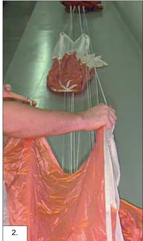
Figure 3. With the slider positioned approximately half way down the suspension lines, flake the canopy in the usual manner.
