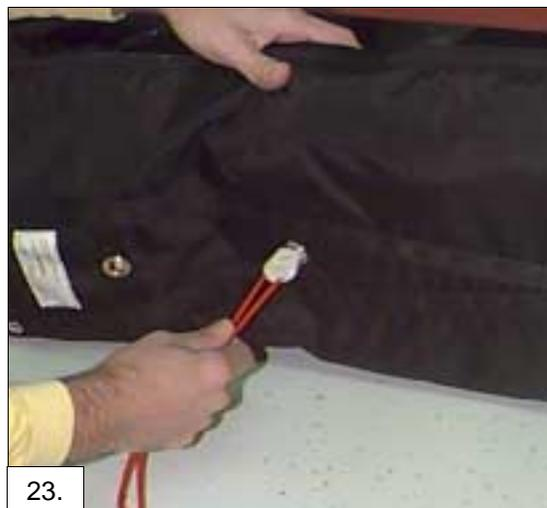
Figure 24. Top of canopy S-folded into the free bag with the first locking pull-up cord in place.
