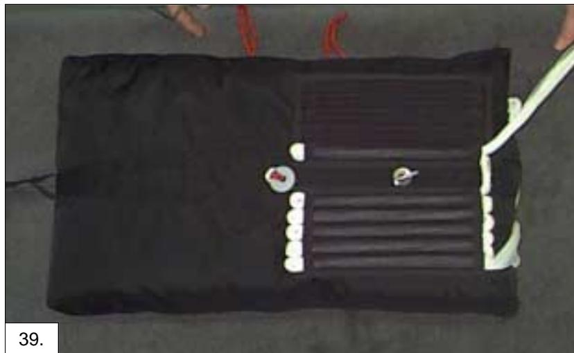
Figure 39. Stow the remainder of the suspension lines in the second set of flutes until you have approximately 12 inches of line remaining between the freebag and the connector links.
