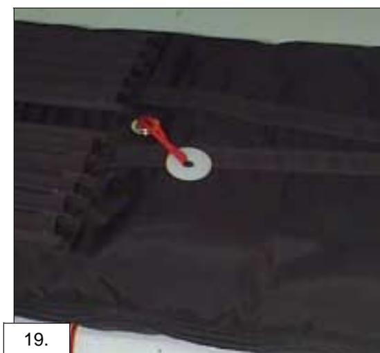
Figure 23. Pull the locking pull-up cord tight and lock in place with the cord-lock.
