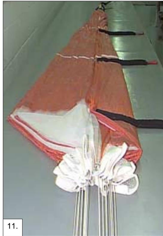
Figure 12. The first folds should generally be to the center without overlap.
