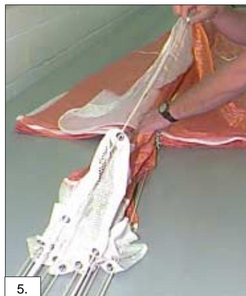
Figure 6. ...and place it into the wind channel of the canopy. Pull the slider apex up as far as it will go, ensuring the slider grommets are against the slider stops on the suspension lines.
