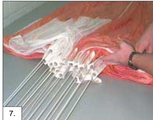
Figure 8. Slider flaked into corresponding canopy gores.
