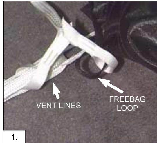
Before placing the canopy into the freebag, there are a few things to keep in mind: the shape of the container, where the pilot chute is going to be placed (upper or lower portion of container), and if the container is Cypres equipped.
