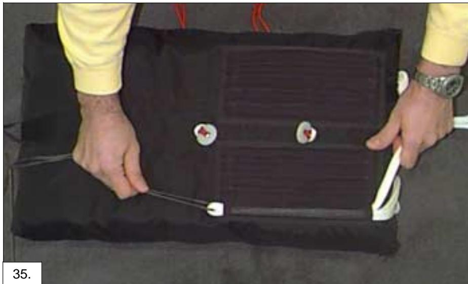
Figure 35. Taking care not to twist the lines, pull the first suspension line bight into the flute.
