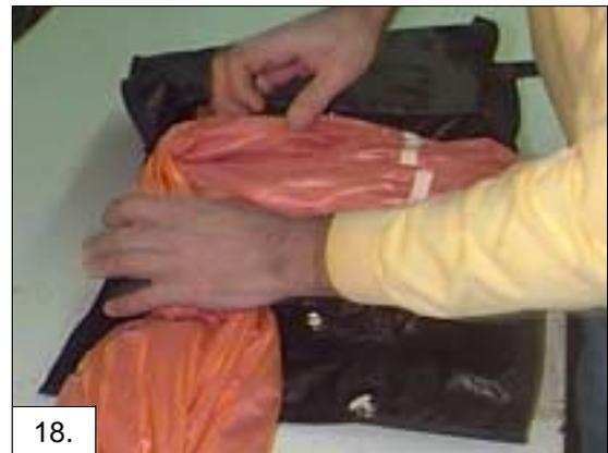
Figure 19. Continue "S" folding the canopy into the freebag.
