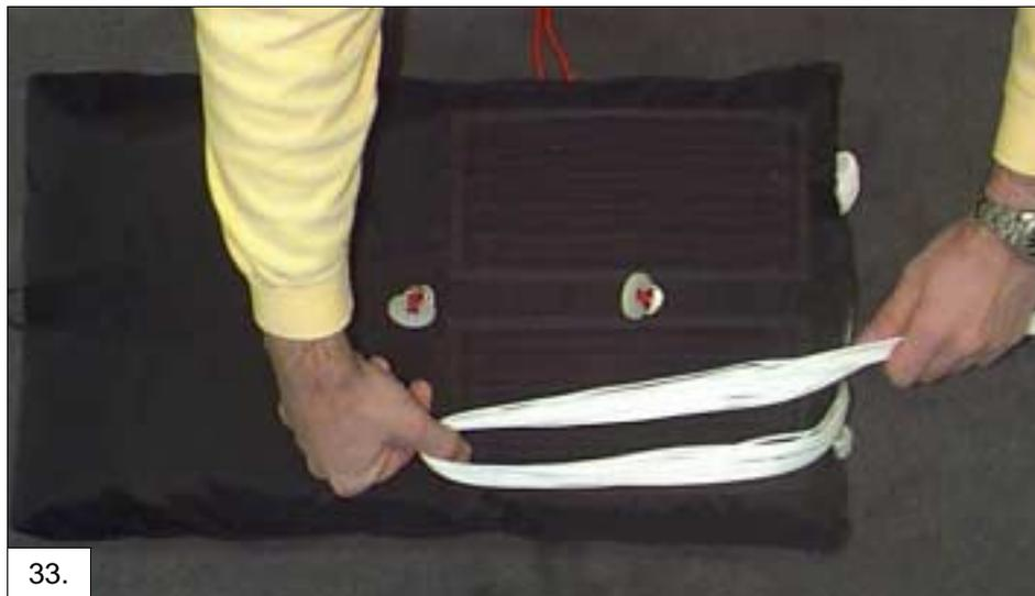
Figure 33. Begin stowing the suspension lines by placing the lines on top of the first stowage flute to measure the correct amount to be stowed. Allow enough for the bight to extend from the top of the flute 1/2" to 3/4".
