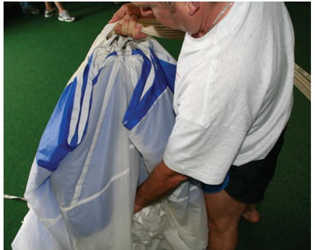
14. Take both sides of the tail in one hand and roll them several times towards the center of the canopy. Pay attention that the canopy fabric stays taut while being rolled, so that it rolls up to the base.
