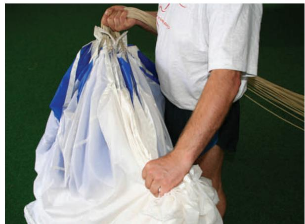
7. Flake out the canopy between line group A and B on each side of the parachute.
