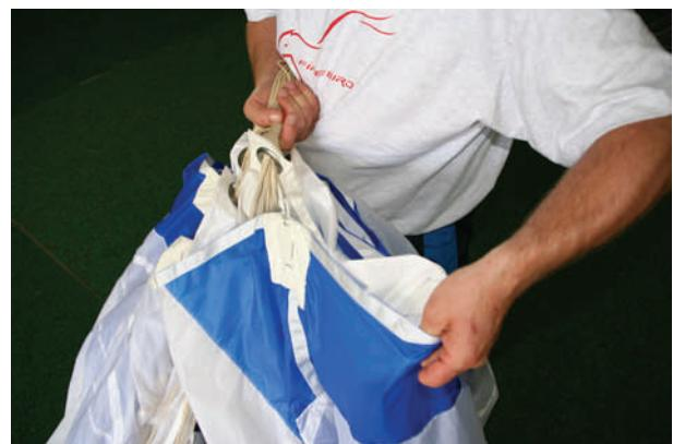
9. Grap all D lines together, pull them out, flake the fabric between C and D lines to the outside and place the D lines in the middle of the parachute next to the slider.
