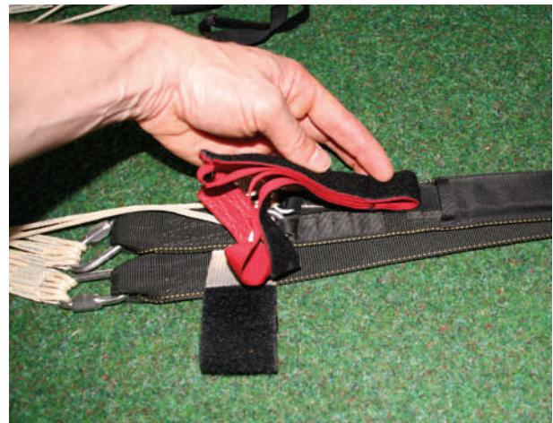
2. At last close the velcro cover of the rear riser tight to keep the toggles in place during the opening.
