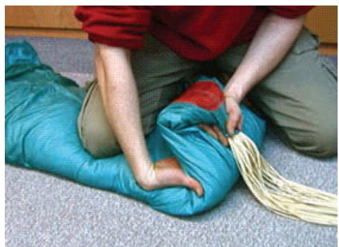
17. Secure the first S-fold with both knees and reach under the cocoon with one hand to compress the material against your thighs. Now fold the upper part of the canopy material over your lower arm and squeeze the rest of the air out, so that it can be folded in an S-fold in the opposite direction from the first S-fold. Continuously secure the canopy material with one hand.
