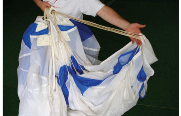
10. Fold the stabiliser onto the lines in the middle.
