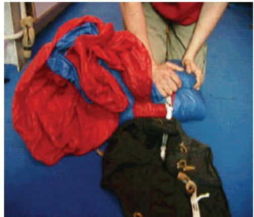
19. Now place the second side into the POD. Secure the canopy with one hand so that it doesn't slip out. How to close the POD and how to put it in the container system please follow the instructions in the manual for the harness container system.
