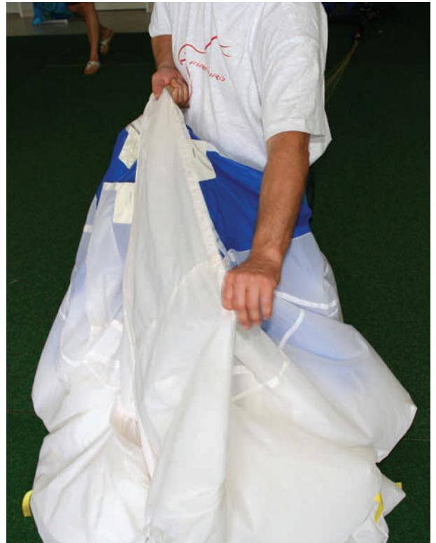
12. The tail is up to the base of the canopy next to the slider grommets.
