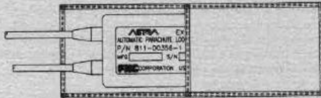
Figure 4 POWER PACK INSTALLATION
