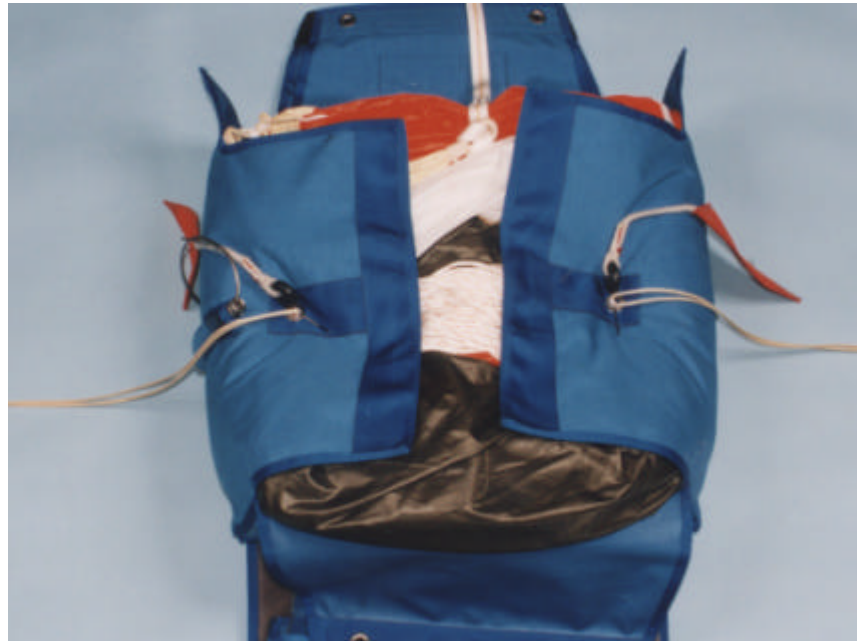
Figure 19 Closing the pack : stage 1
