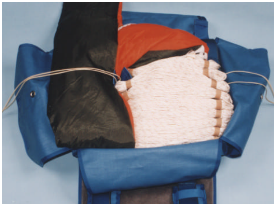
Figure 14 Stowing the canopy : stage 1
