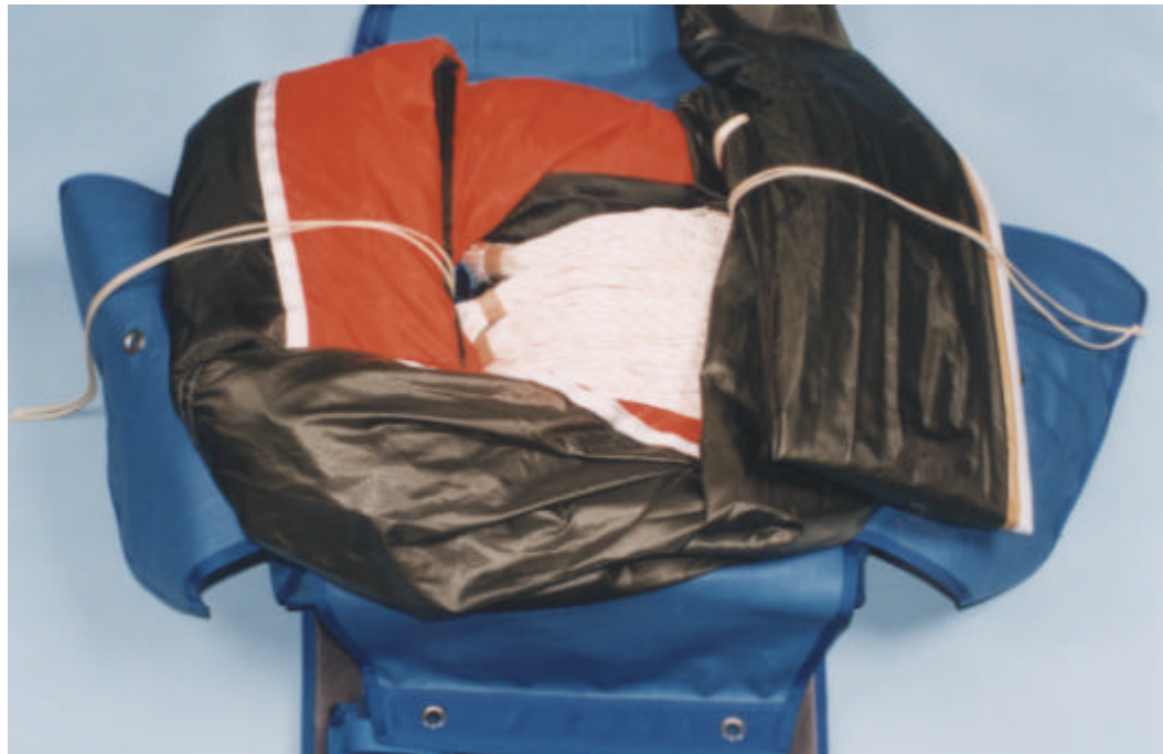
Figure 16 Stowing the canopy : stage 3
