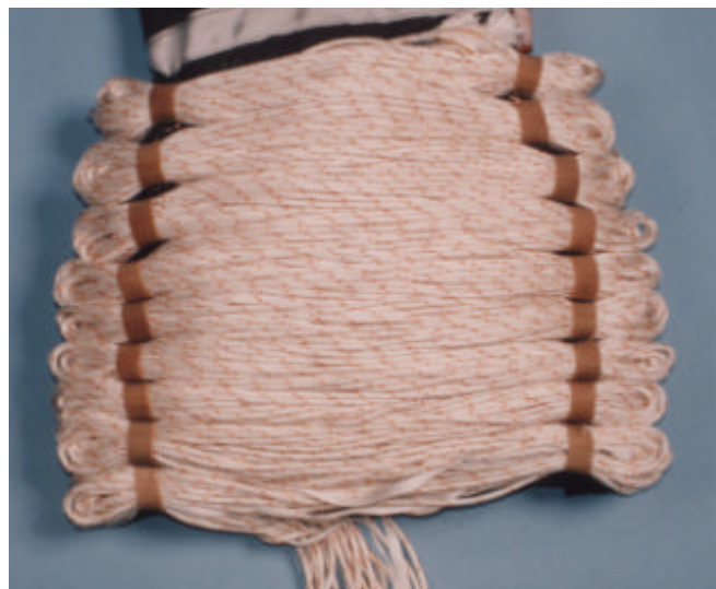
Figure 10 Diaper closed rigging lines stowed
