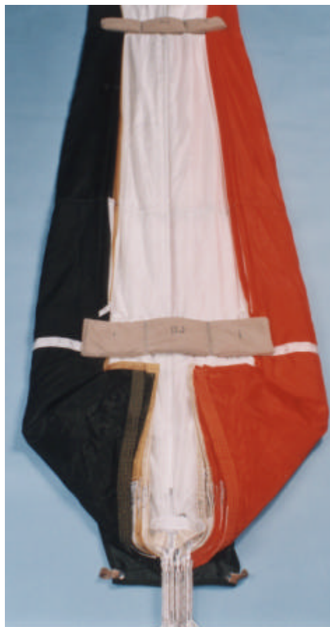
Figure 6 Folding the canopy : stage 1
