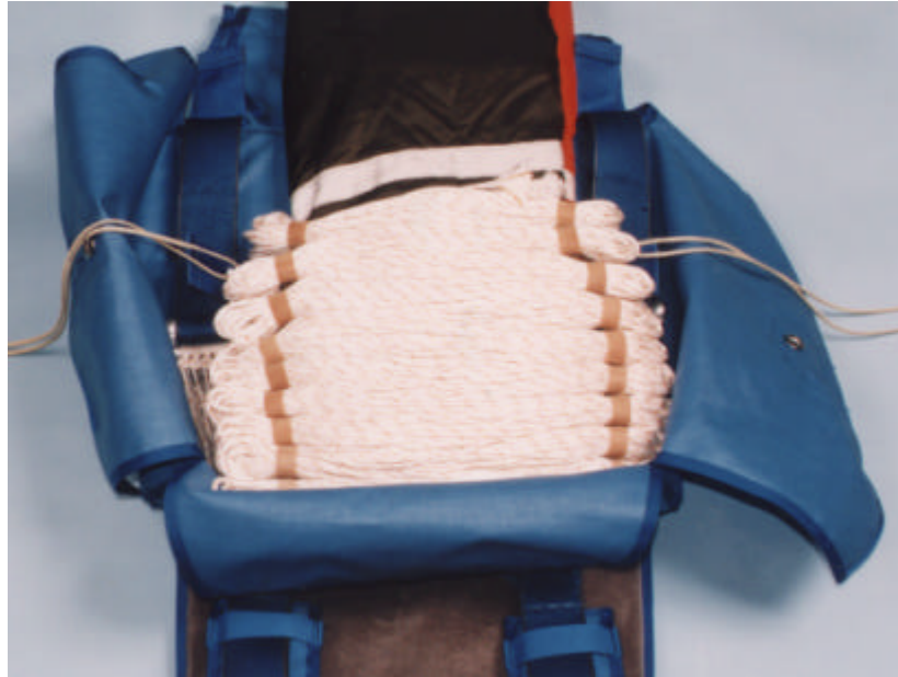
Figure 13 Risers and diaper positioned in pack
