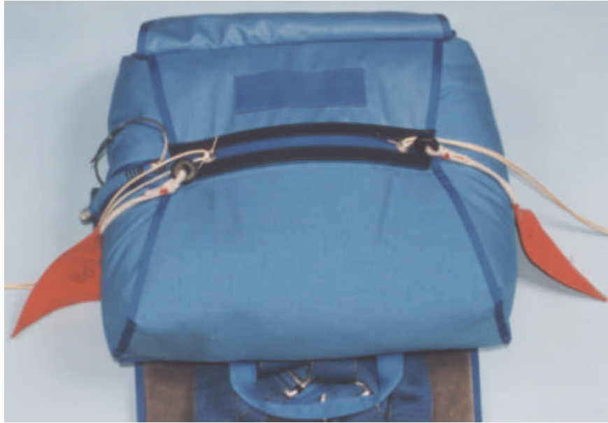
Figure 23 Closing the pack : stage 3
