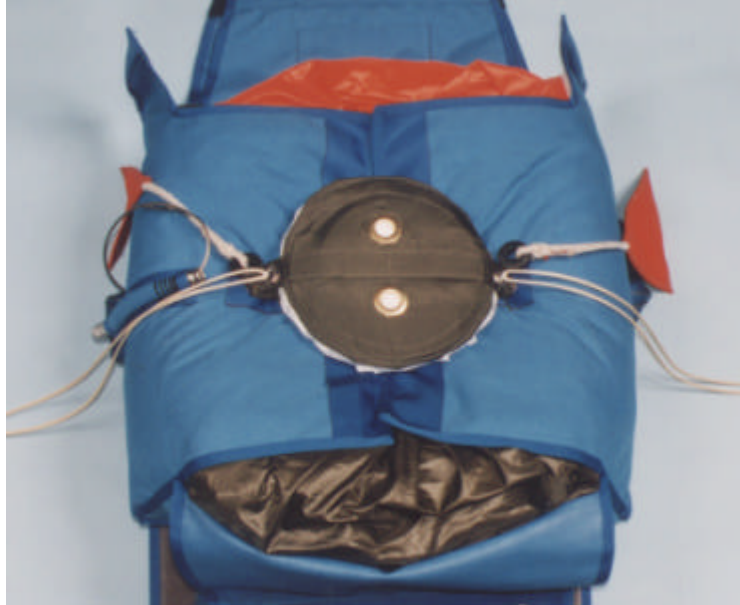
Figure 21 Pilot chute secured
