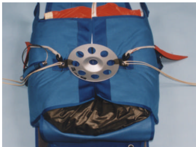
Figure 20 Positioning the kicker plate
