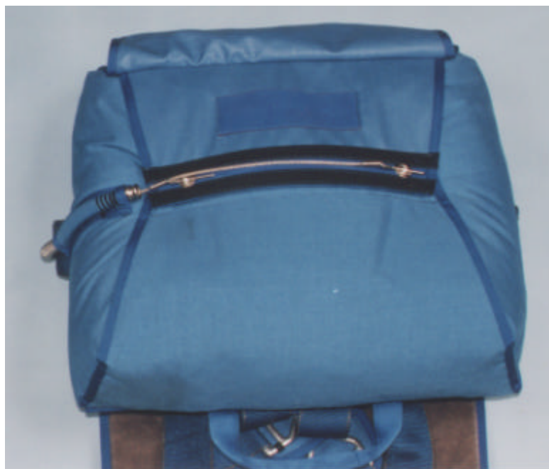
Figure 24 Pack closed ripcord pins fitted
