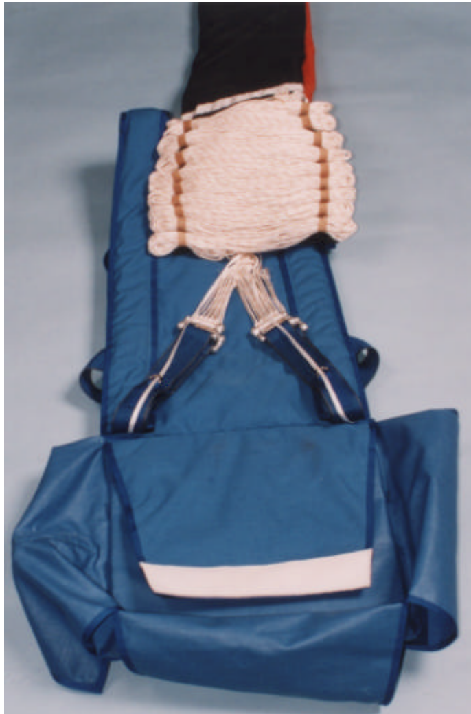
Figure 11 Riser covers secured
