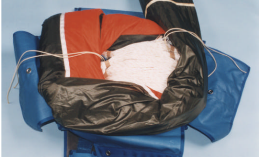
Figure 15 Stowing the canopy : stage 2
