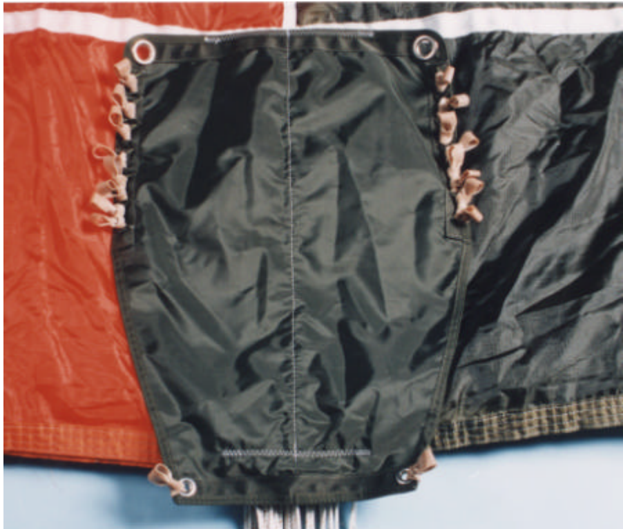
Figure 2 Attaching the connecting line and pilot chute
