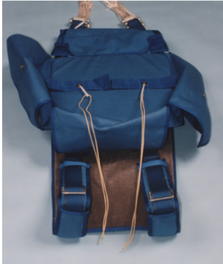
Figure 12 Fitting the closure loop
