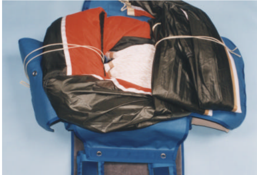
Figure 17 Stowing the canopy : stage 4
