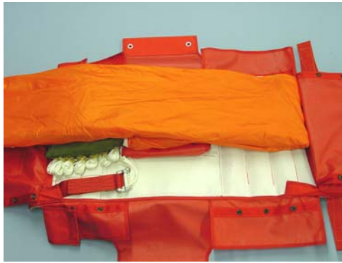
Fig 18 Stowing the canopy : 1st fold
