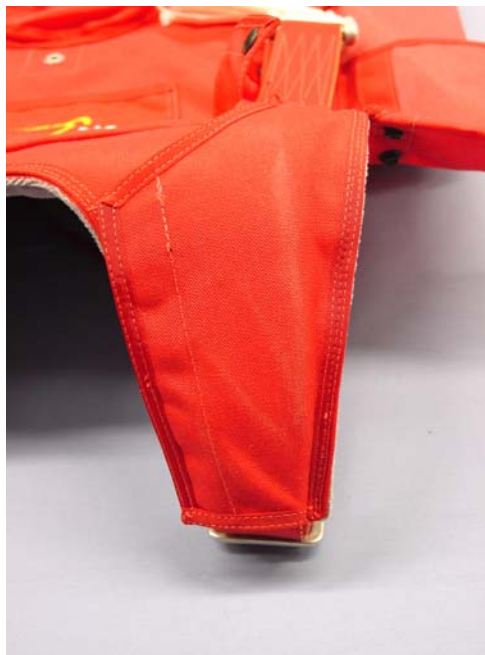
Fig 14 Lift webs positioned in covers
