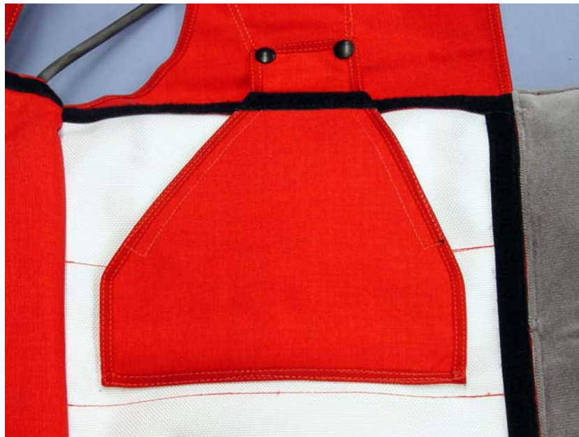
Fig 31 Ripcord pins in position
