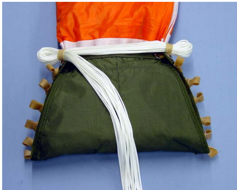
Fig 11 Closing the diaper : stage 1
