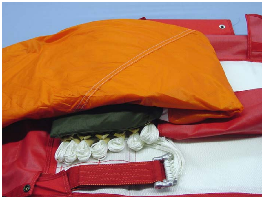
Fig 16 Lift webs positioned
