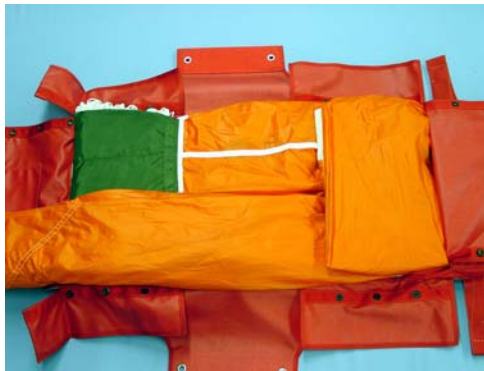
Fig 18 Stowing the canopy : 1st fold
