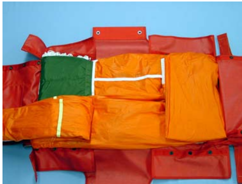
Fig 19 Stowing the canopy : 2nd fold
