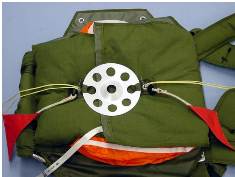
Fig 19 Closing the container : stage 1
