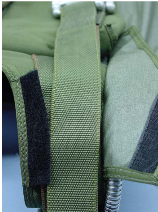
Fig 12 Diaper closed rigging lines stowed
