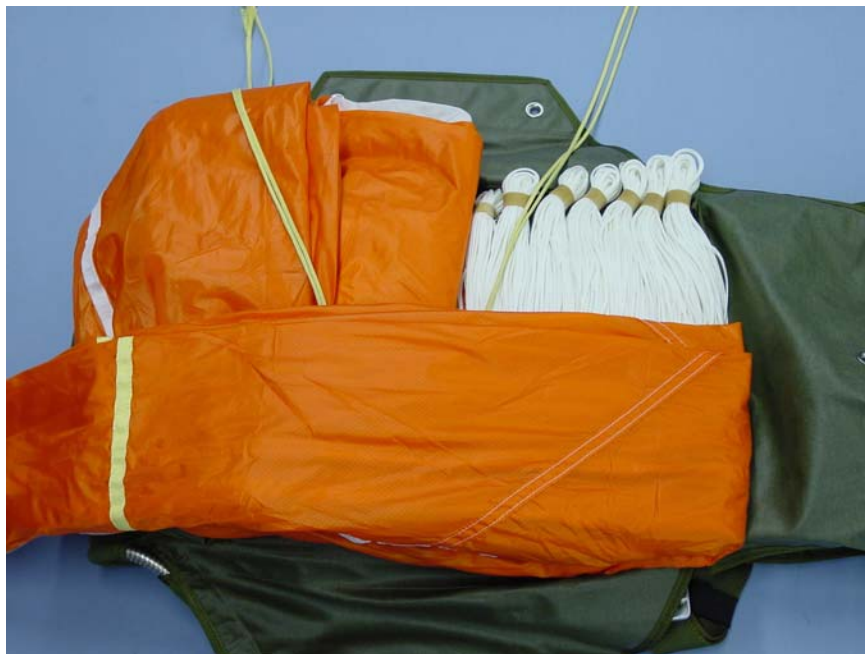
Fig 16 Stowing the canopy : first fold
