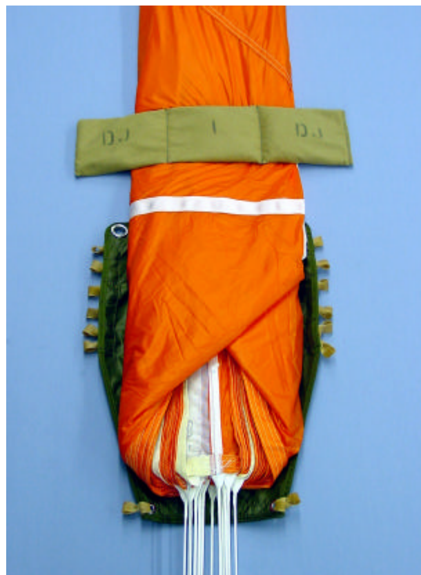
Fig 9 Folding the canopy – stage 2
