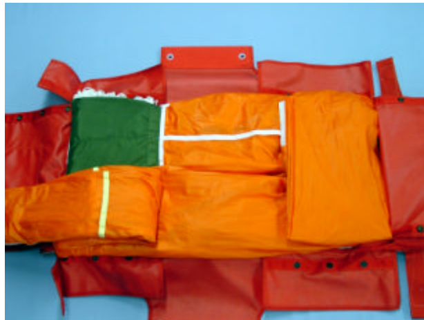
Fig 19 Stowing the canopy : 2nd fold
