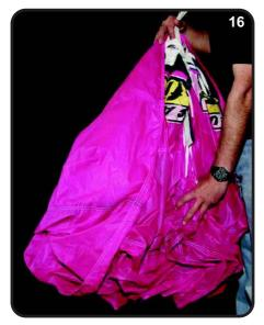
Reach down and pick up the center of the parachutes tail, where the warning label is sewn on. Raise the tail just above the slider and hold it in place with the same hand that is holding the lines. Now start on one side to pull the excess material straight out and wrap that part of the tail half way around the canopy. Repeat that procedure on the other side of the parachute in the same manner.
