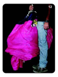
Since all the lines are bunched up in the middle, pull each stabilizer panel out one by one until they form an irregular shape and be sure that none of the lines are wrapped around a slider stop on a stabilizer.
