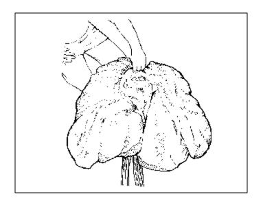
**L.** Tuck the re main der of the can opy un der the bundle un til it is the height of the bag.
