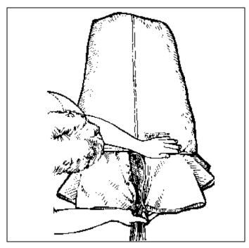
**I.** Fold the ex posed sta bi liz ers back un der the tail. Lay your hand 6"-8" from the bot tom of the bun dle and fold the can opy back over it self.
