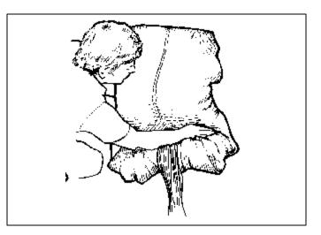
**K.** Fold the can opy back over so you now have an 8" S- fold at the bot tom. The length and number of S- folds may vary ac cord ing to the distance be tween the ver ti cal part i tion that sepa rates the main and reserve con tain ers, and the grom met in the bot tom flap of the reserve con tainer.
