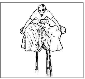
**H.** Re turn the cen ter tail tab to the bot tom cen ter of the bun dle. Where the sta bi liz ers at tach to the main body of the can opy. "Co coon" the can opy to the width of the bag.
