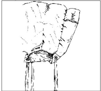
NOTE: The pur pose of the flag is to cover the nose during de ploy ment and for the pock ets on the flag to in flate and hold the flag in place cov er ing the nose and slow ing in flation.
