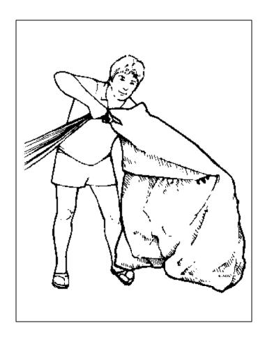
**E.** Kneel at the top of the can opy fac ing the container. Draw the can opy to ward you while at the same time nar row ing the bun dle to the width of the bag. Con stantly work the fab ric away from the links.
