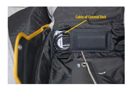
The cables must not be stowed in the pouch determined for the device body, nor shall they be stowed (partially) under the device body. There is a risk of damaging the cables. Stow the cutter and the control unit in accordance with the Manual provided by the container manufacturer so that in both cases there is at least minimum space for the cables. Space for cables reduces the change of damage to the device after packing and during normal use.
