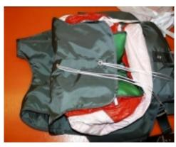
Route lower pull up cord through the grommet in the bottom flap and keep the flaps together by knotting the pull up cords together.
