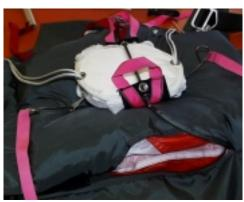
Pull up both closing loops with the pull up cords and secure with flagged temporary closing pins.
