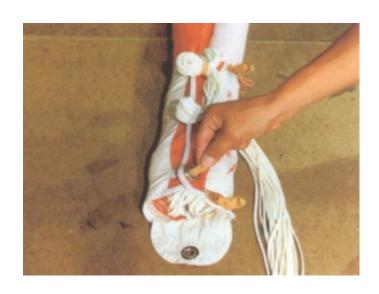
Close the bottom flap on top of both side flaps using a line loop of no more than 4 cm.
