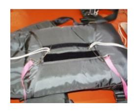
While you hold the closing loop with the pull up cord and the tightening tools, you remove the top temporary closing pin. Carefully install one of the S-hooks in the closing loop.
