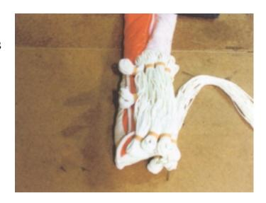
It is mandatory that the pilot chute bridle be installed through both positioning loops on 2 apex vent lines and around all the other vent lines. It must have a stitching through the loop to prevent the bridle from tightening around the vent lines.
