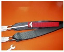
Short loop to be put on the top ripcord pin. Long loop to be put on the end ripcord pin.
