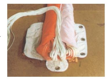
Form a loop of suspension lines. No more than 3-4 cm. Close the diaper starting with the top rubber band through the top grommet. Continue with the centre grommet.
