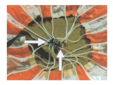
With a fixed wrench size 9 check that connector links are tightened. Never over tightened.
