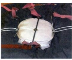
Close left side flap and secure with the temporary closing pins.
