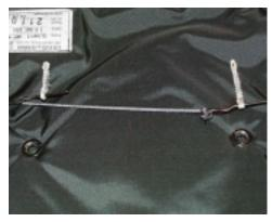
Lead both loops through each their grommets in the bottom of the container. Put a pull up cord in each loop.
