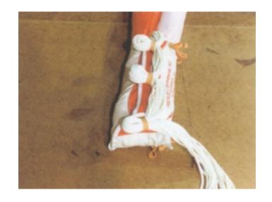
Finish stowing of the remaining suspension lines lengthwise using loops of no more than 4 cm
