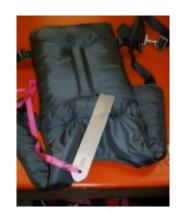
Flip over the container and check that both ripcord pins are correctly in place.
