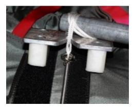
Slowly and carefully remove the pull up cord from the loop. You form this pull up cord into a large loop with a slip knot. Place this large loop in the other S-hook.
