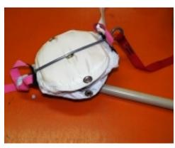
S-fold the pilot chute bridle cord and place it in the valley between the grommets.
