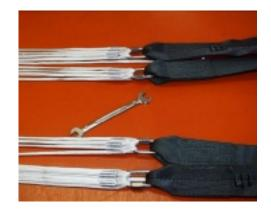
Check that toggles are in correct place on the Velcro.
