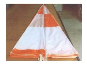
Align the skirt band and up fold 45° parallel with the main seams.
