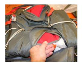
The pilot chute bridle cord is routed out under top flap.
