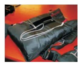
Put the large loop around your knee or foot to be able to expand the spring with your leg.
