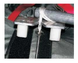
Slowly and carefully remove the pull up cord from the loop. Form a 2m long pull up cord into a large loop with a slip knot. Place this large loop in the other S-hook.
