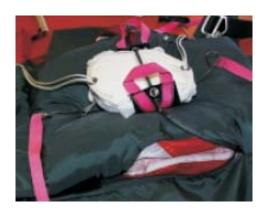
Left hand Side flap is secured with the temporary pins.
