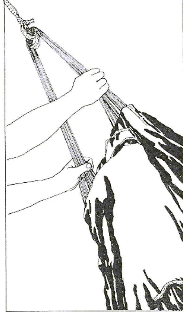
Examine the suspension lines for entanglements by taking the lines from the top center gore (#1 and #24) in one hand and from the bottom center gore (#12 and #13) in the other, then following them down from the skirt to the risers.
