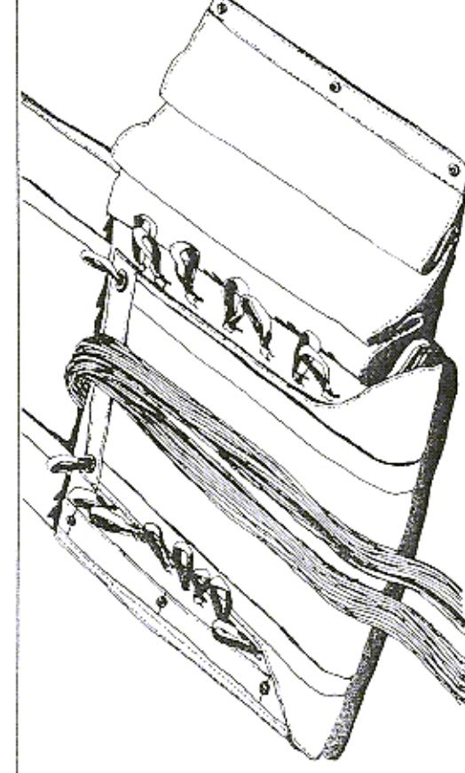
*Note:* The lines will appear uneven because the tension on the control lines makes them shorter. Compensate for this unevenness during stowing by taking a slightly longer length of suspension lines than control lines for each stow.
