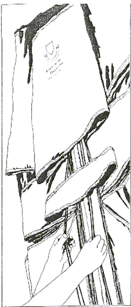
Fold the outside edges of the pleated gores inward on each side until the width of the canopy is slightly less than that of the sleeve. Pull down the sleeve to the stabilization panels (figure 13).
