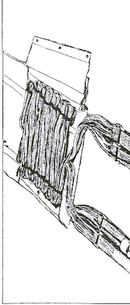
Fold the locking flap into position and bring the retainer bands through the flap grommets. Stow the first loop in the left-hand retainer, then the second loop in the right-hand one (figure 16).
