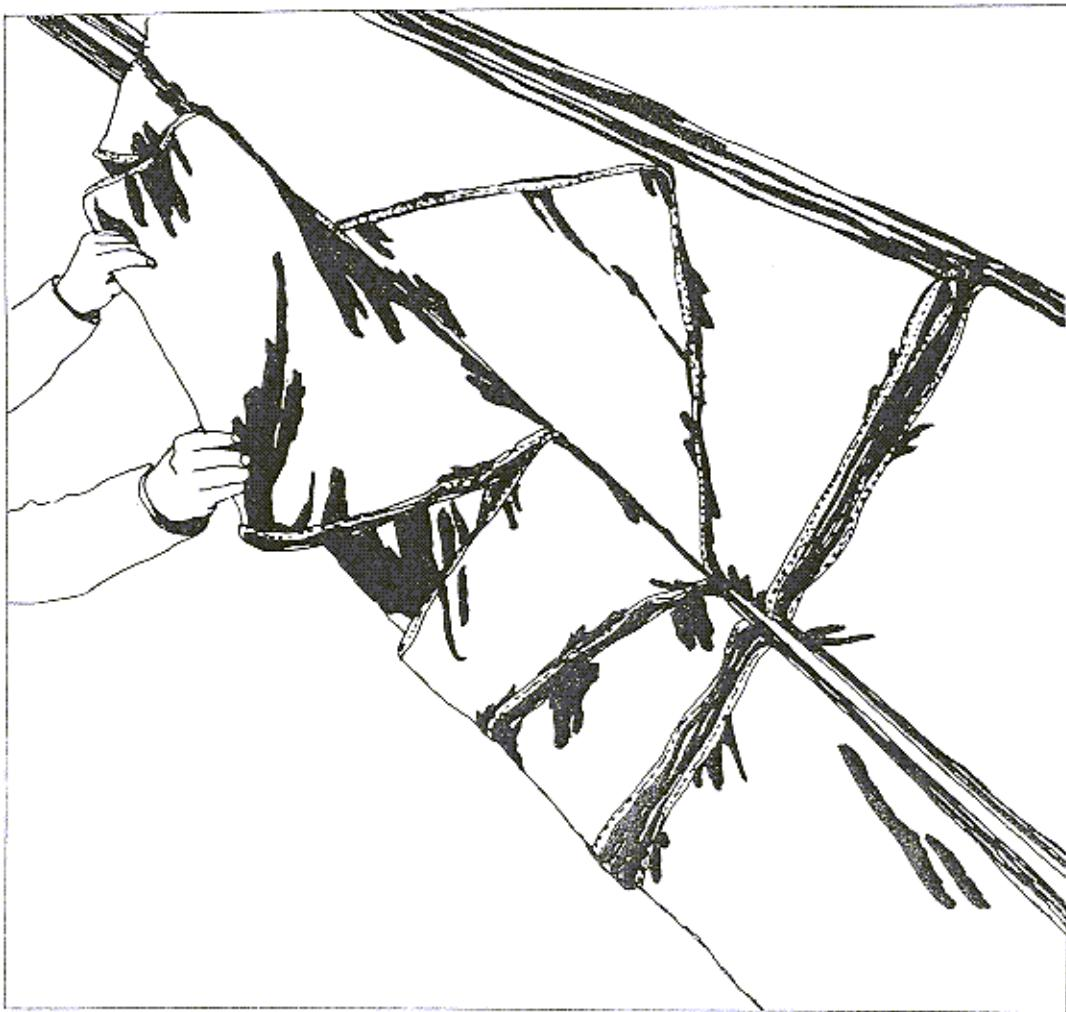
Note: Make sure that the top of the canopy is pulled out from and clear of the crown lines and that all the material at each slot is pulled out of the center channel. Unusual slackness or tightness of one or more suspension lines indicates an entanglement in the upper part of the canopy.
