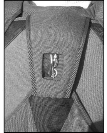
Access to breakaway and reserve ripcords, main opening system as well, are fully free and easy to be grabbed. FXC control unit (if used) is free of access as well.
