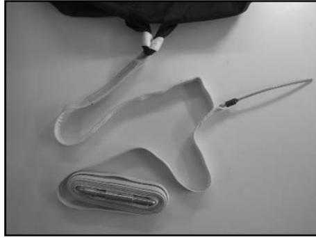
Static line must be route to the left side of the main container before closing it. The main container is secured with the cable installed on the static line.
