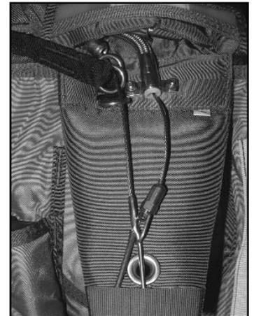
Install the A.A.D. main unit into its pocket, cable connexion must be facing downward. **Airtec installation kit is only allowed for Cypres A.A.D. type.** Stow remaining cables and route the cutter and the control unit in the white type 4 /1.5" channel toward the collar.
