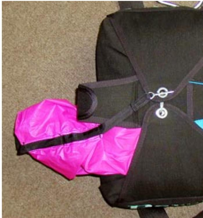
**Close the side flaps and make sure, that there is enough pilot chute fabric still outside of the container, that you have a non restricted connection between your pad and the pin.**
