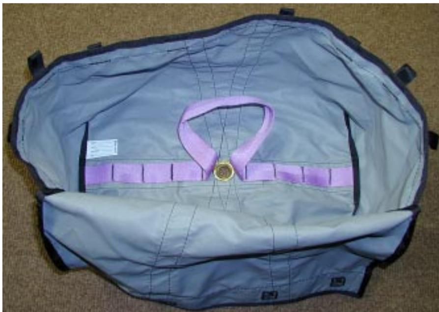
The main deployment bag features a special loop, which allows the instructor to easily change from freefall mode to static line mode by simply pulling the loop to the other side of the bag where it attaches to the static line. See pictures on next page.
