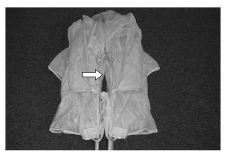
**14)** Quarter the slider, dividing the material evenly between the slider grommets. Make sure the slider grommets are seated against the slider stops sewn into the stabilizers.
