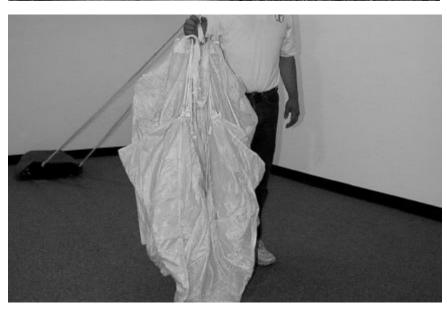
**4)** Starting with the end cell nearest your legs, begin flaking the nose of the canopy. Pull each cell completely out, and keep it in your hand. Then, pick up the next, taking care not to miss any until all seven cells are in your hand.
