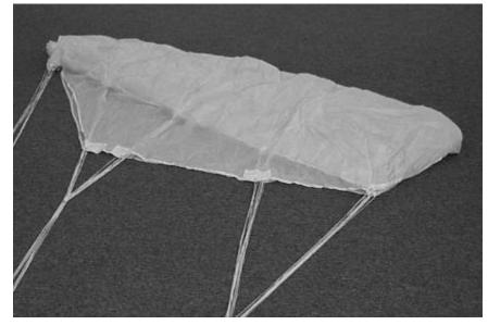
2) Crouch next to the risers and face the canopy. Be sure there are no twists in the risers. Slip the fingers of your left hand between each left hand riser and between the left hand steering line and the risers. Do the same with your right hand. Slide your fingers up onto the lines as shown, grasping the lines below the slider.
