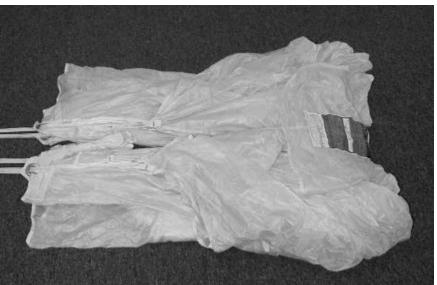
7) Starting on the right side of the canopy, carefully lift the folds of material back towards the center of the pack job until the nose is exposed. Clear the three cells to the right of the center cell and flake this section of the nose toward the outside of the pack job.
