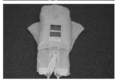
**17)** Carefully S-fold the nose under the canopy, making sure the leading edge remains exposed, but does not extend past the edges of the folded canopy.
