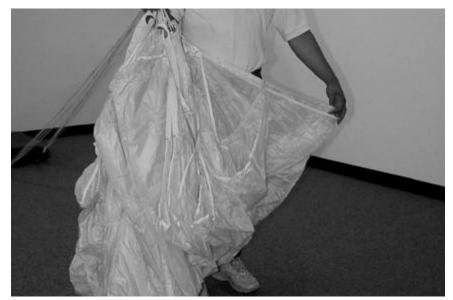
5) Clear the stabilizers. Flake the material between each line group out toward the stabilizers, keeping the line groups stacked together in the middle of the pack job. Clear the tail, flaking the material between each steering line toward the outside of the pack job.
