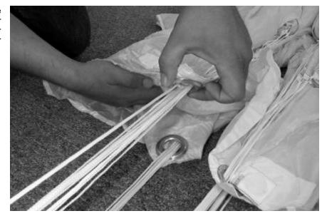
**15)** Dress the center of the tail by spreading out the top center panel to the width of the canopy underneath.
