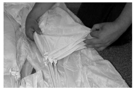
**13)** Repeat steps 7 through 12 to flake and the left side of the canopy. Make sure the line channel in the center of the pack job is clear, as indicated by the arrow in the picture at right.
