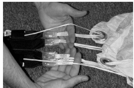
3) Start moving up the lines, allowing them to slide between your fingers. Push the slider ahead of you until you reach the bottom of the canopy. Carefully lift the canopy off of the ground. Make sure the lines are not twisted and the canopy is facing the correct direction. The nose openings should be facing the rig, and the tail should be farthest from the rig.
