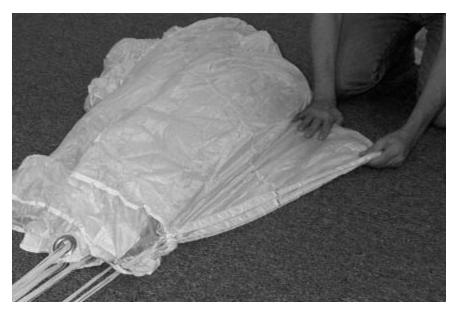
**8)** Flake the material between the A and B lines away from the line channel in the center of the pack job. Be sure that all three T seams to the right of the center cell are neatly flaked.
