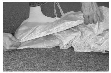
**9)** Find the four bottom seams to the right of the center cell and flake them out toward the stabilizer. The bottom seams are where the loaded ribs meet the bottom skins.
