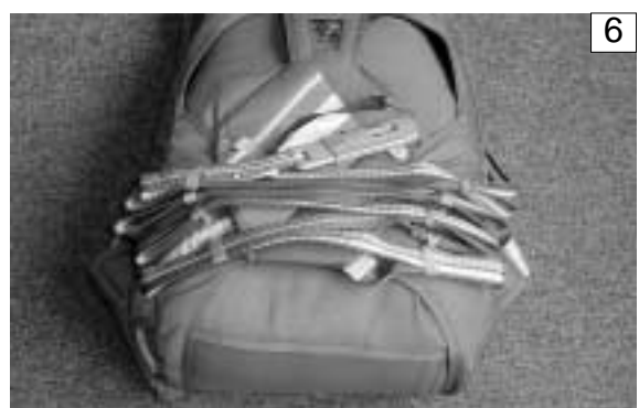
6 Fermer le rabat de protection, lover la S.O.A. sur les élastiques prévus à cet effet. Close the protective flap, stow the static line in its rubber bands located on the two lateral flaps.
